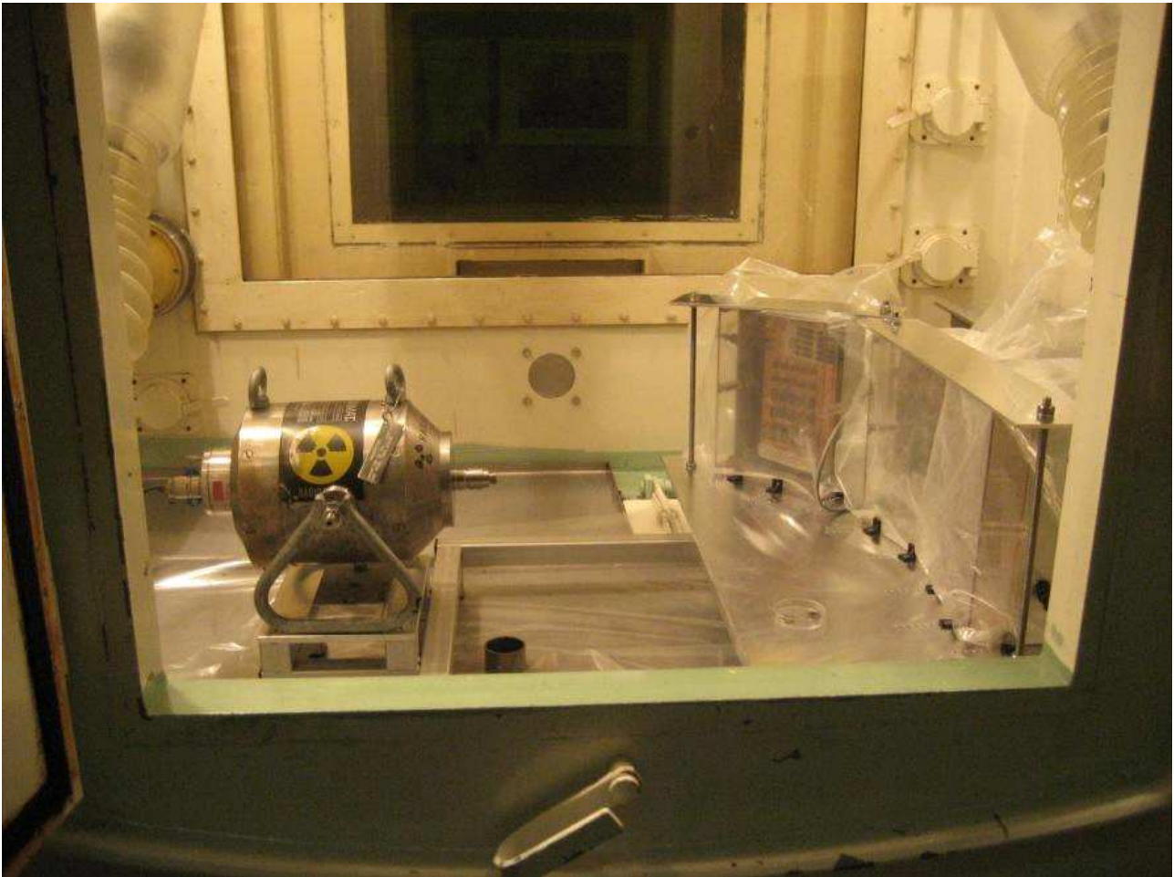
Figure 2: Low dose rate facility; on the left side the radiography camera is positioned, on the right side up to three boxes can be mounted that house one PCB each. The PCB used for the experiments reported here is mounted in the leftmost box.
