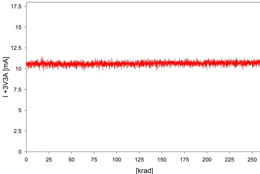
Figure 5: Analog supply current of the MFA104 (3.3 V analog)
