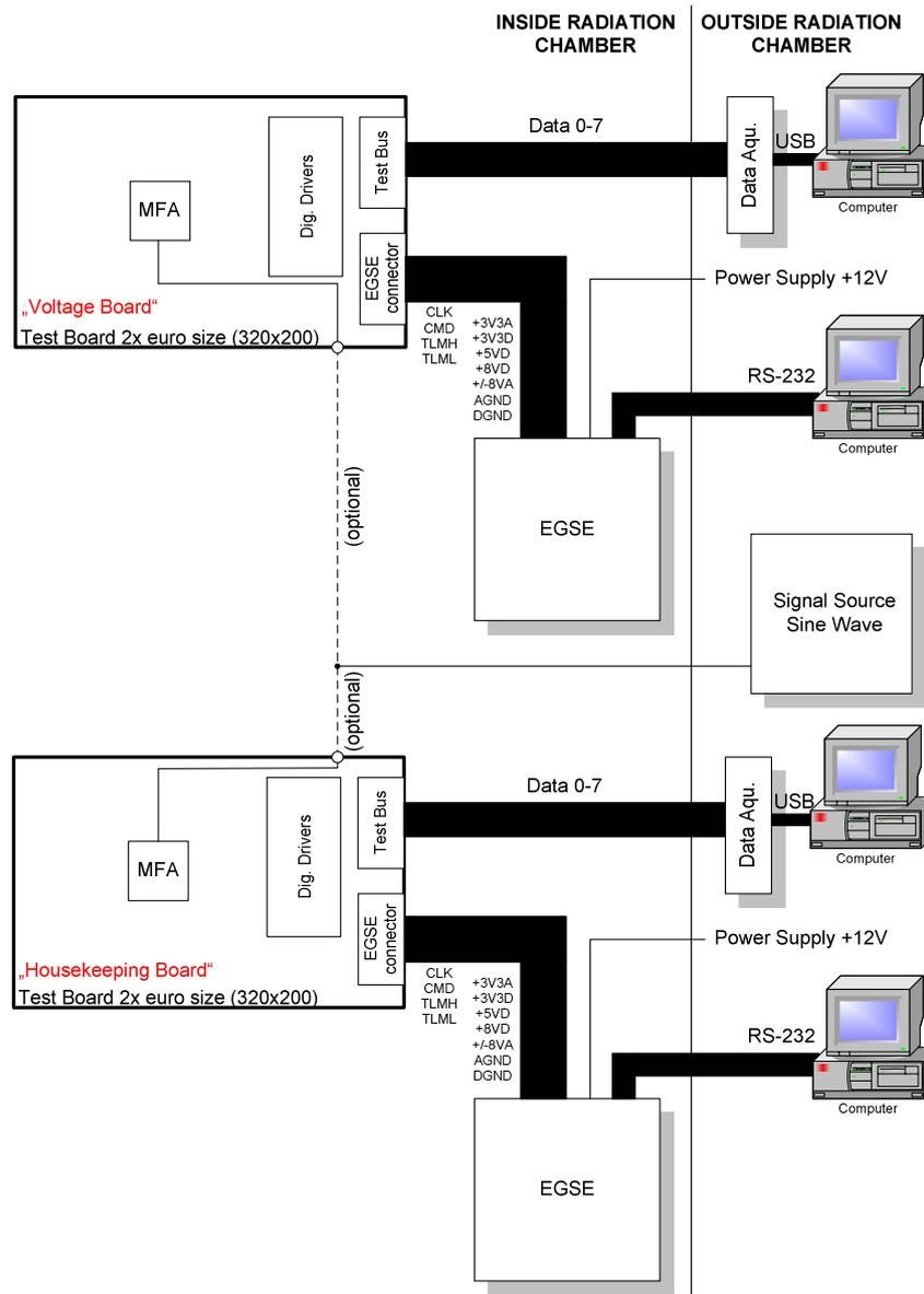
Figure 2: Test configuration
