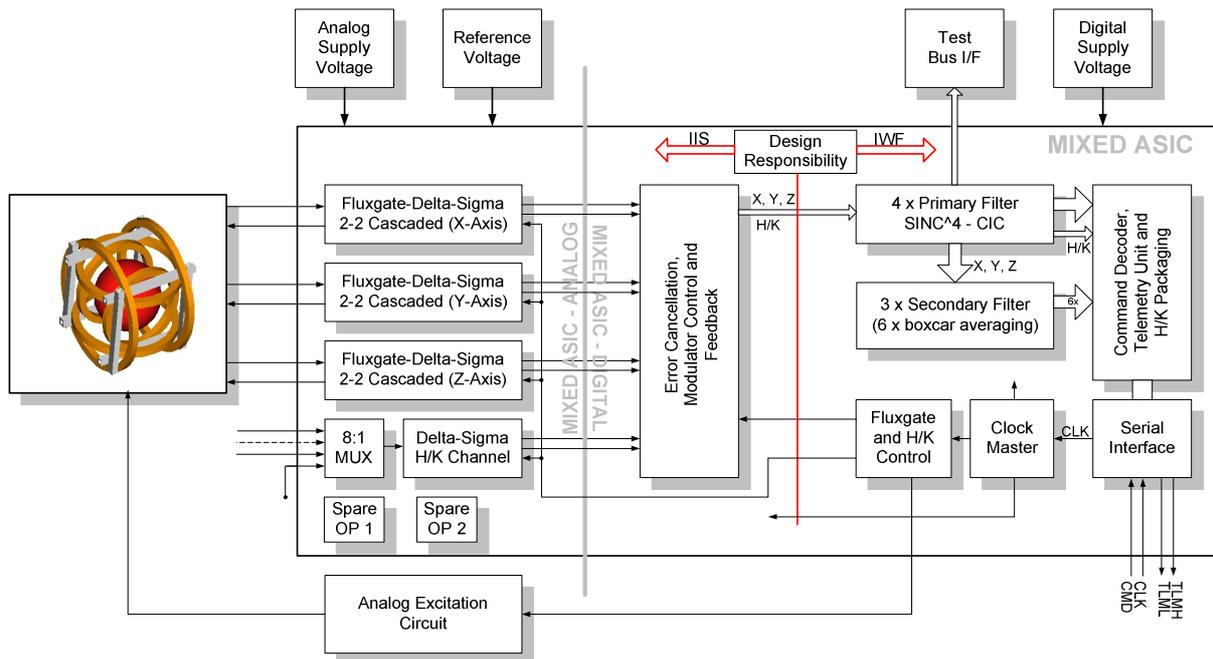
Figure 1: Top level block diagram of the MFA
