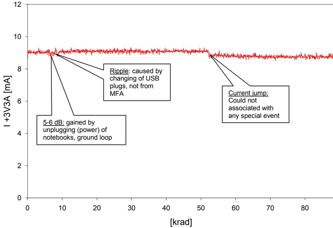
Figure 15 Analog supply current of the MFA109 (3.3 V analog)
