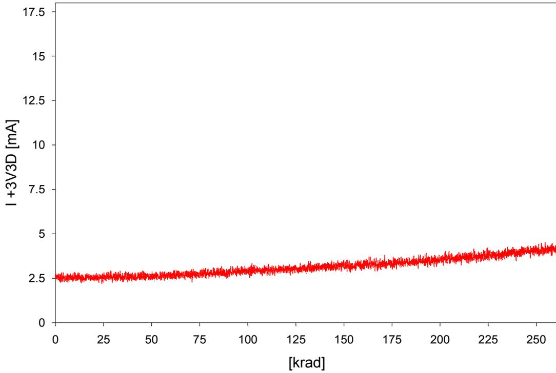
Figure 6: Digital supply current of the MFA104 (3.3 V digital)
