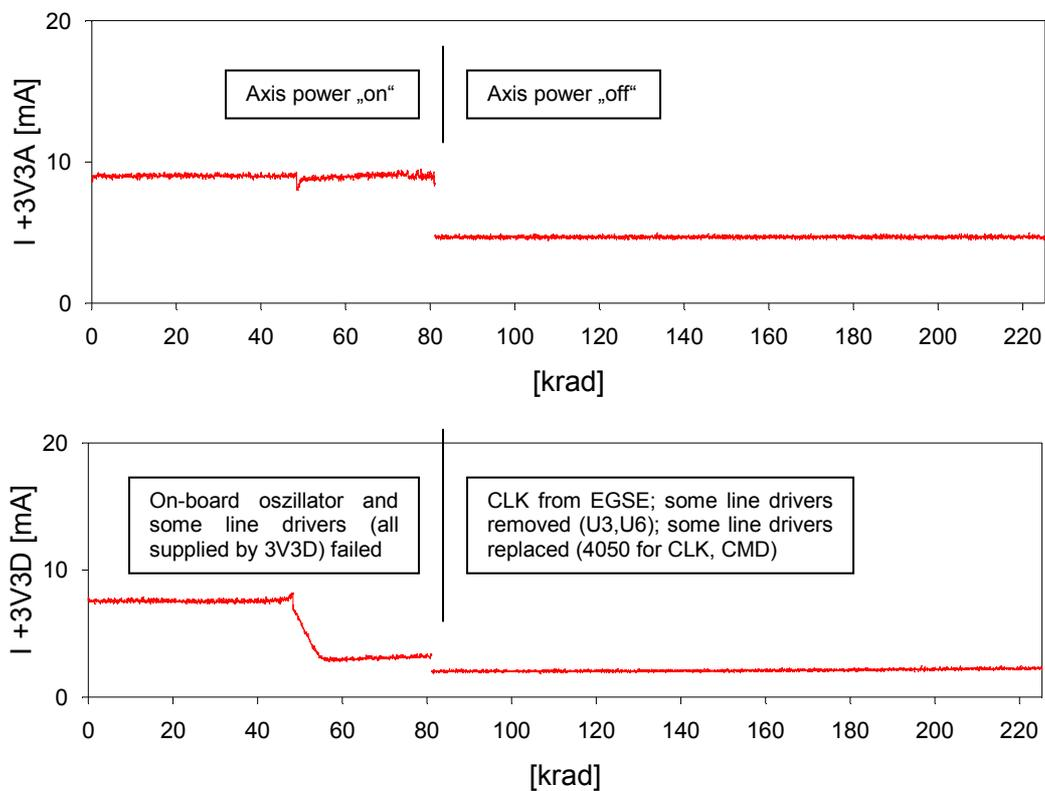
Figure 12: Digital (lower) and analog (lower) supply current of the MFA112
