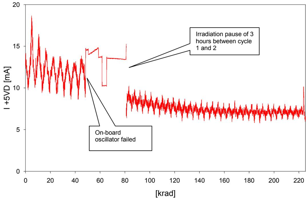
Figure 13: Digital supply current of the test board (5 V digital)
