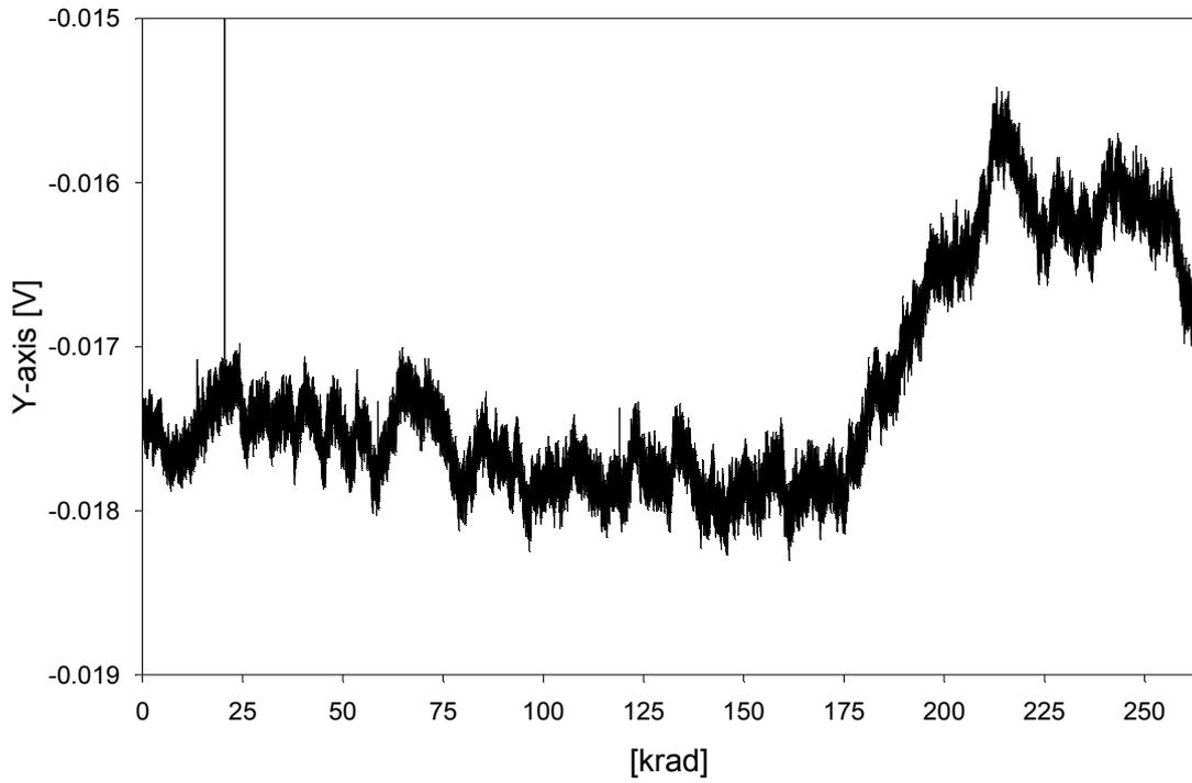
Figure 8: Low telemetry (1.5 Hz) output of the short circuited Y-axis
