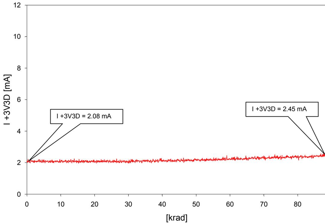
Figure 16 Digital supply current of the MFA109 (3.3 V digital)
