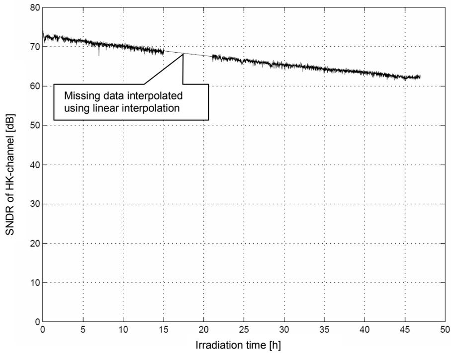
Figure 10: SNDR of the differential housekeeping channel
