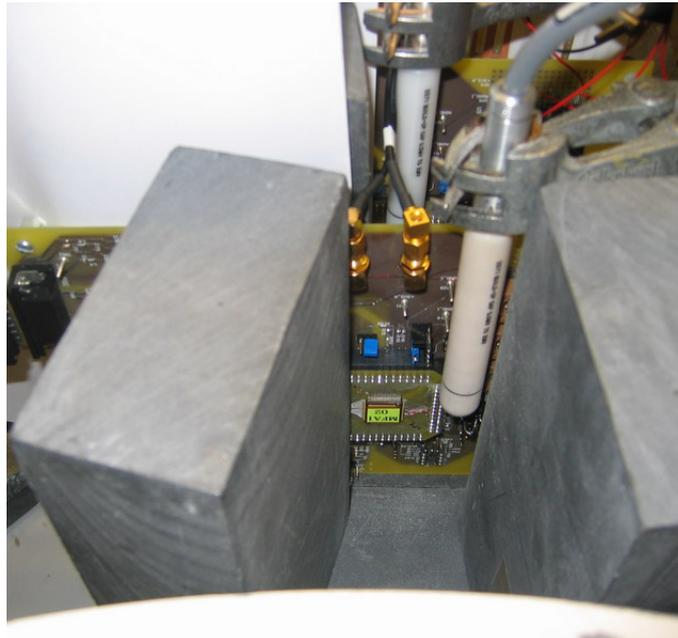
Figure 4: Adapter board of the MFA with the dosimeter above it
