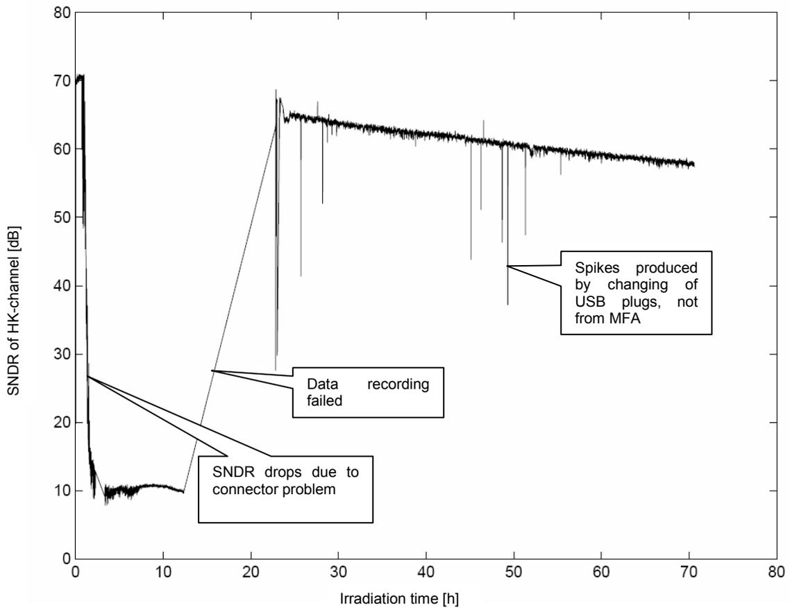
Figure 14: SNDR of the differential housekeeping channel
