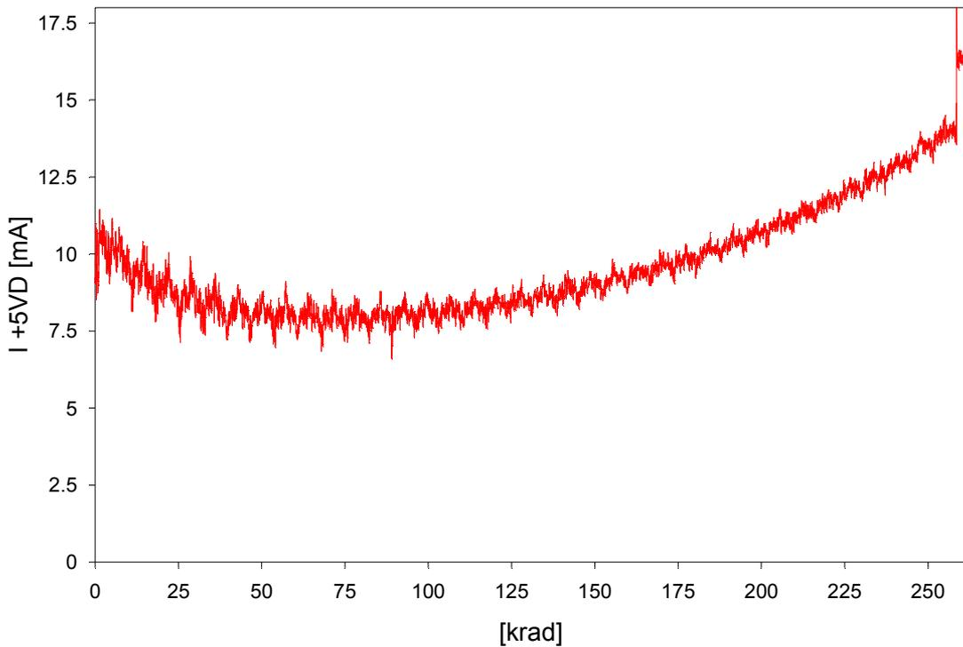
Figure 7: Digital supply current of the test board (5 V digital)
