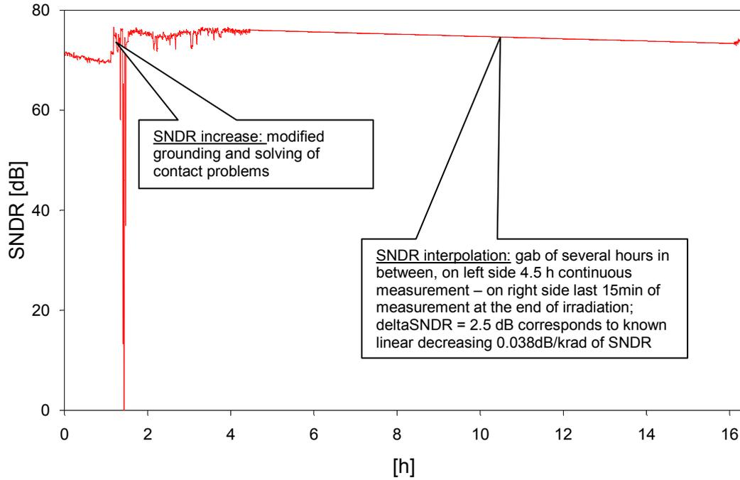
Figure 17 SNDR of the differential housekeeping channel
