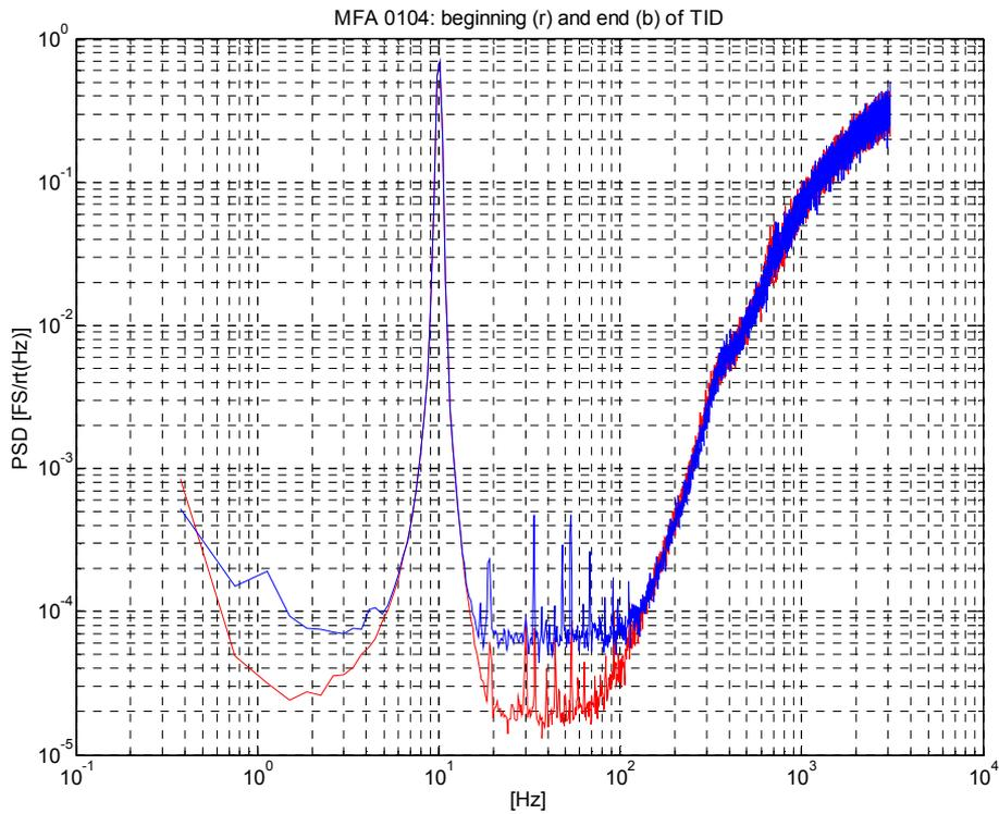
Figure 11 Power spectral density of the diff. H/K channel: beginning (red) and end (blue) of 261.5 krad test
