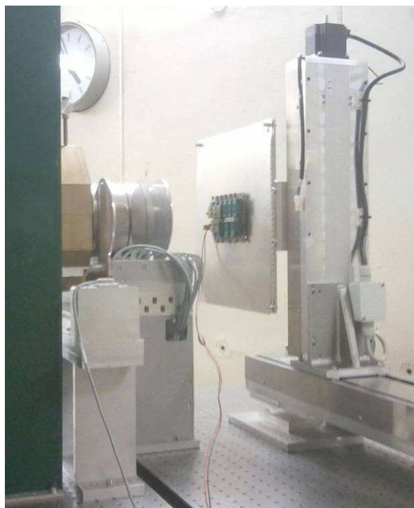
Figure 5: samples installed for irradiation
