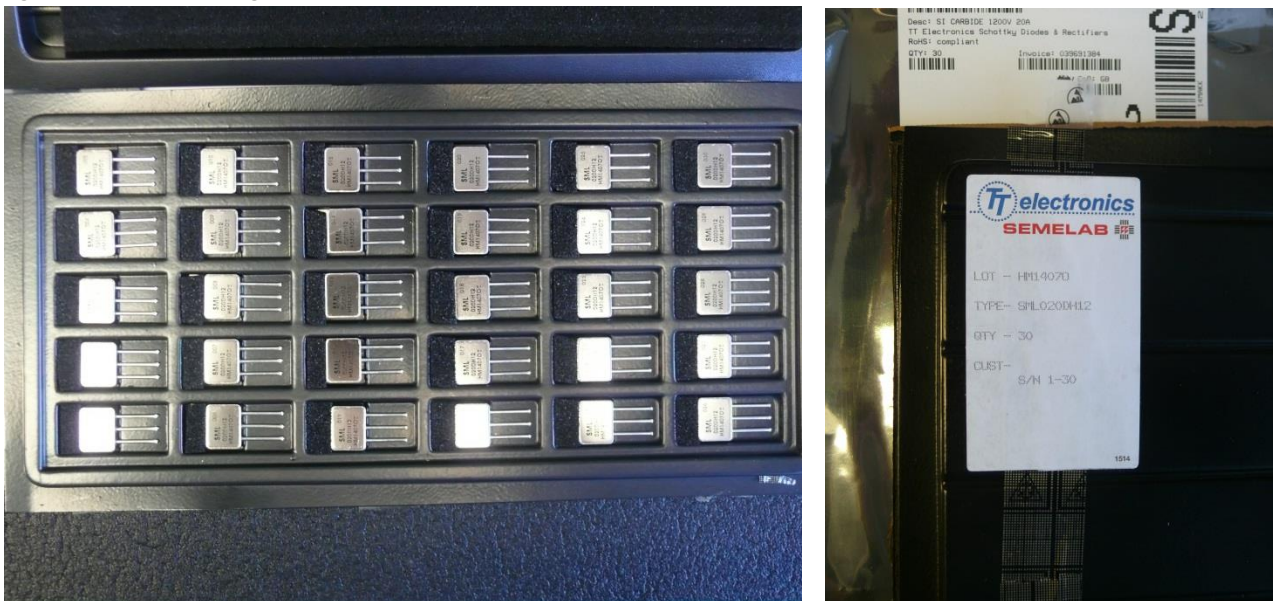
Figure 2: The ESD package with the samples
