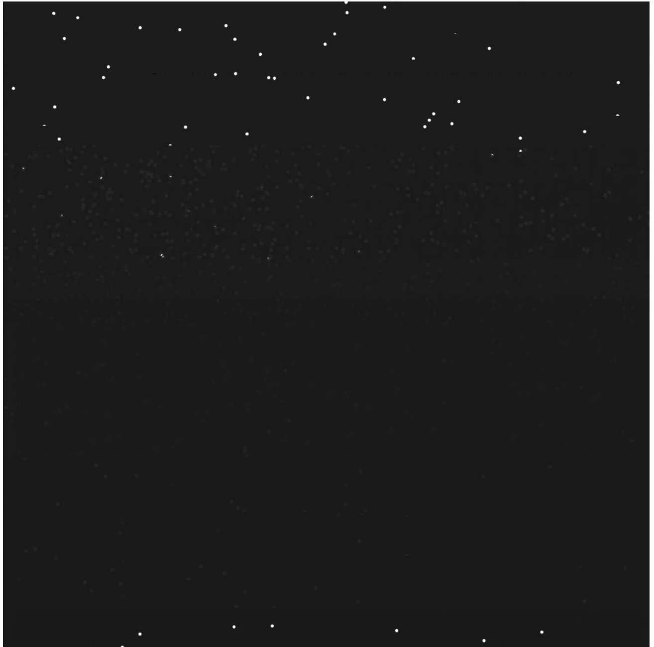
Figure 7-6 : Image acquired under ^{83}\text{Kr}^{25+} ion beam at 0^\circ in DR mode with 16 ms integration time and addressing per frame operation –several corrupted areas observed
