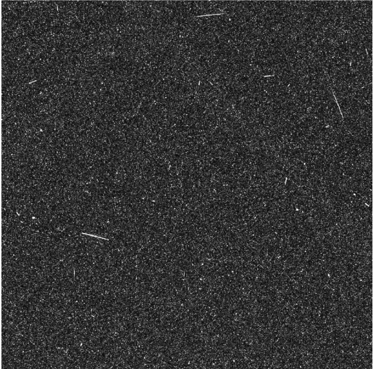
Figure 7-3 : Typical full frame final image acquired under 230 MeV proton flux with 200 ms integration time in addressing per frame NDR mode
