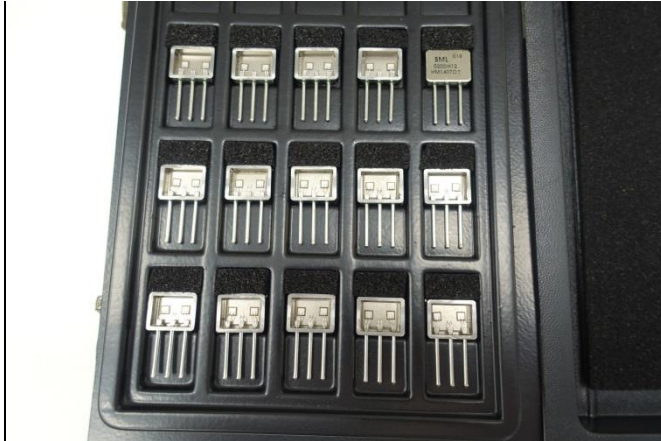
Figure 5: DUT decapsulation. Batch of decapsulated SML020DH12
