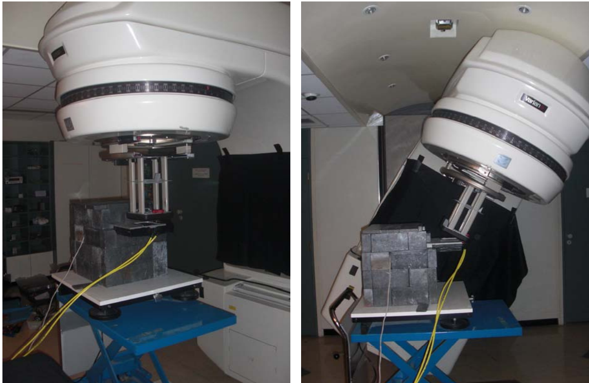
Figure 5-6 : Test bench irradiated with a normal (left) and 28.2° tilted (right) electron beam
