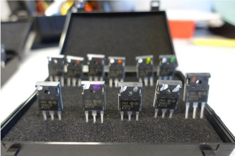
Table 4: Sample marking: Due to a limited number of samples, the DUTs tested with protons were previously used for a 1 Mrad(Si) TID campaign. Only DUTs used in the tests of this report are shown.
