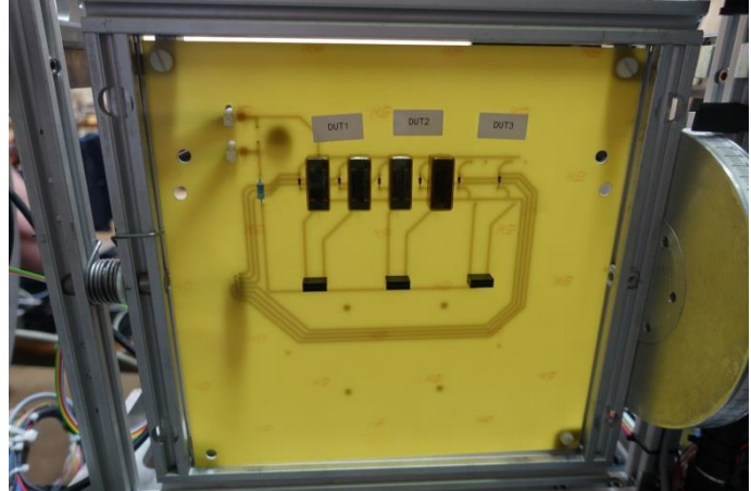
Figure 10: Test board layout Top left side: proton tests at JULIC, top right side: Heavy ion tests at UCL, bottom left: Heavy ion tests at GANL
