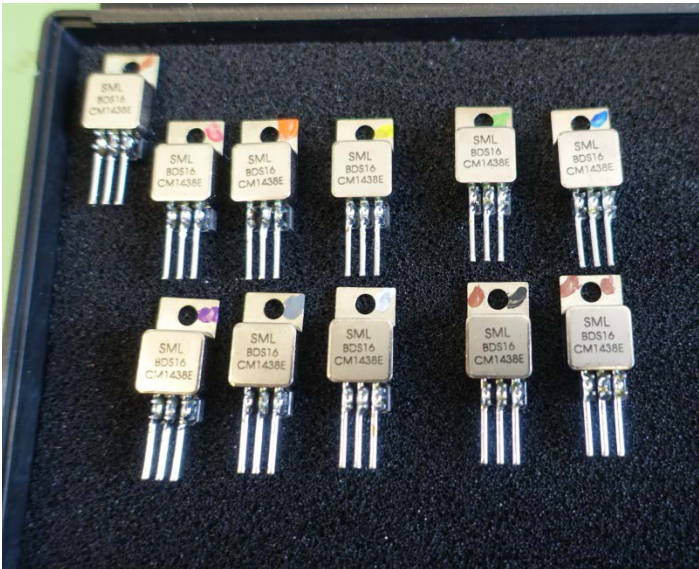
Figure 4: Sample marking. Top image: LDR-Test, bottom image: HDR-Test.
