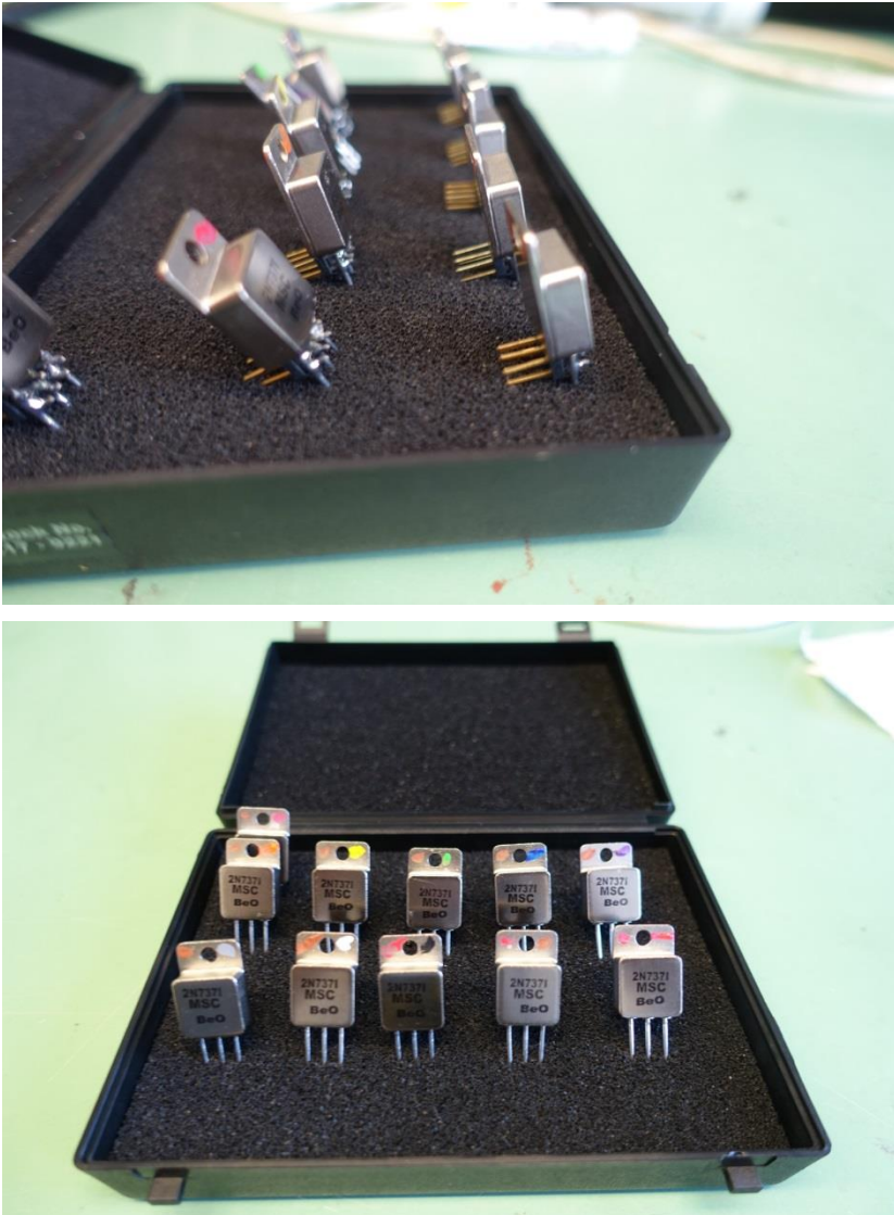
Figure 4: Sample marking. Top image: LDR-Test, bottom image: HDR-Test. The images are exemplary as they show the similarly prepared 2N7371 in the identical package.
