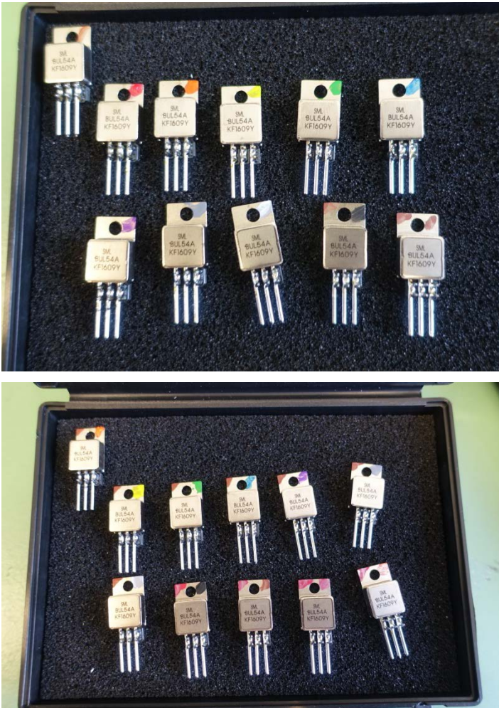
Figure 4: Sample marking. Top image: LDR-Test, bottom image: HDR-Test.
