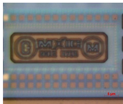
Figure 4: Die marking (top die).
