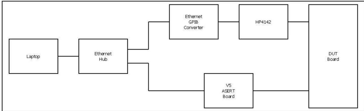
Figure 4 - Test set-up block diagram
