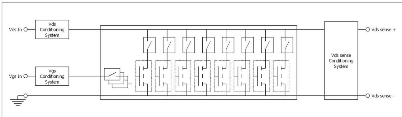
Figure 5 - DUTs board - One line schematic
