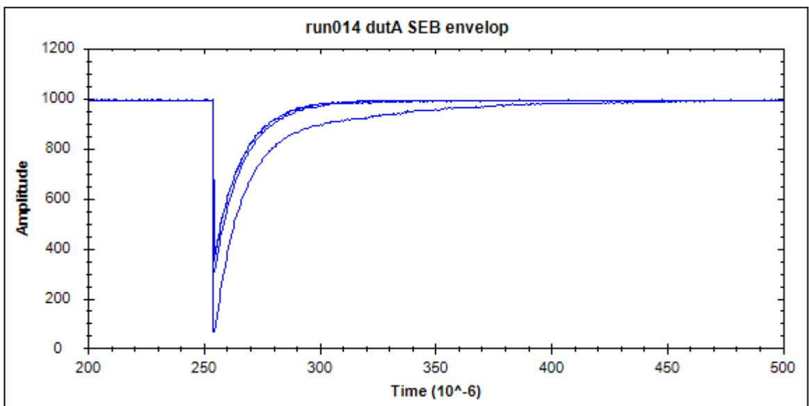
Amplitude is measured in tester LSBs (1 LSB correspond to 307mV)
