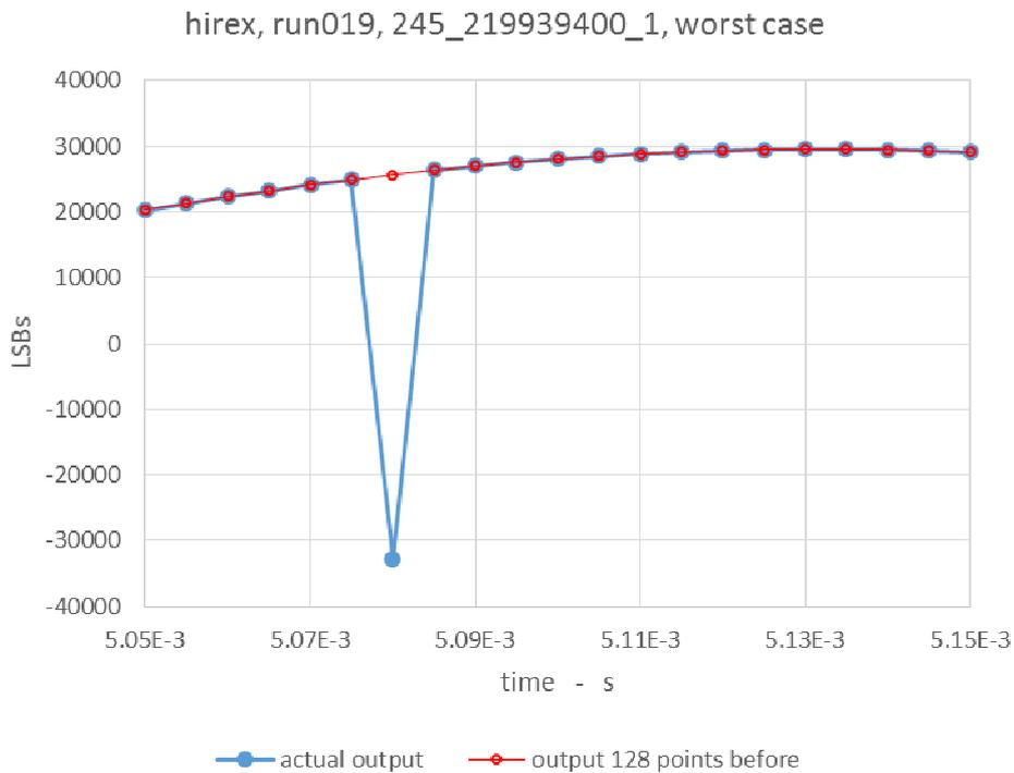
Figure 10 – W35, run039, worstcase single conversion error (error amplitude is 58440LSBs)
