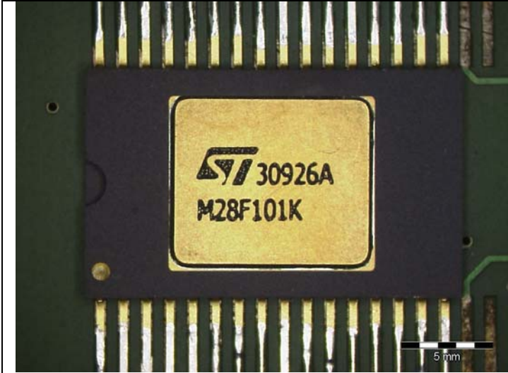
Photo 1 – Device Top marking
