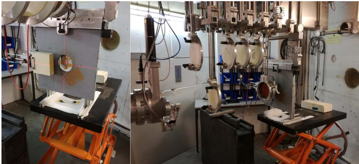
Figure 3-5 Irradiation setup of the proton radiation. (Left picture) Alignment of the fiber spool to the center of the proton beam. (Right picture) Complete irradiation setup: On the left is the accelerator's exit, in the center the degraders to adjust the energy of the protons and to the right is the fiber under test (not visible here). Photographs by UCL.
