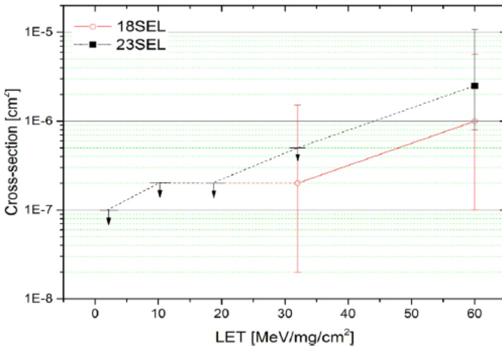
Figure 3-34 Micro-lachup cross-section for Marvell at 1Gb/s and heat on.
