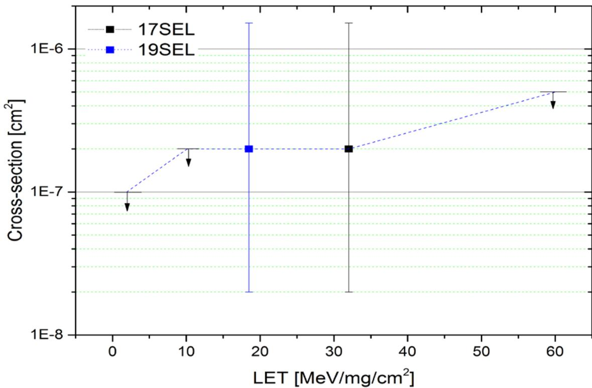
Figure 3-42 MicroLatch-Up" cross-section for Vitesse components at 1000 Mb/s mode (heat on).
