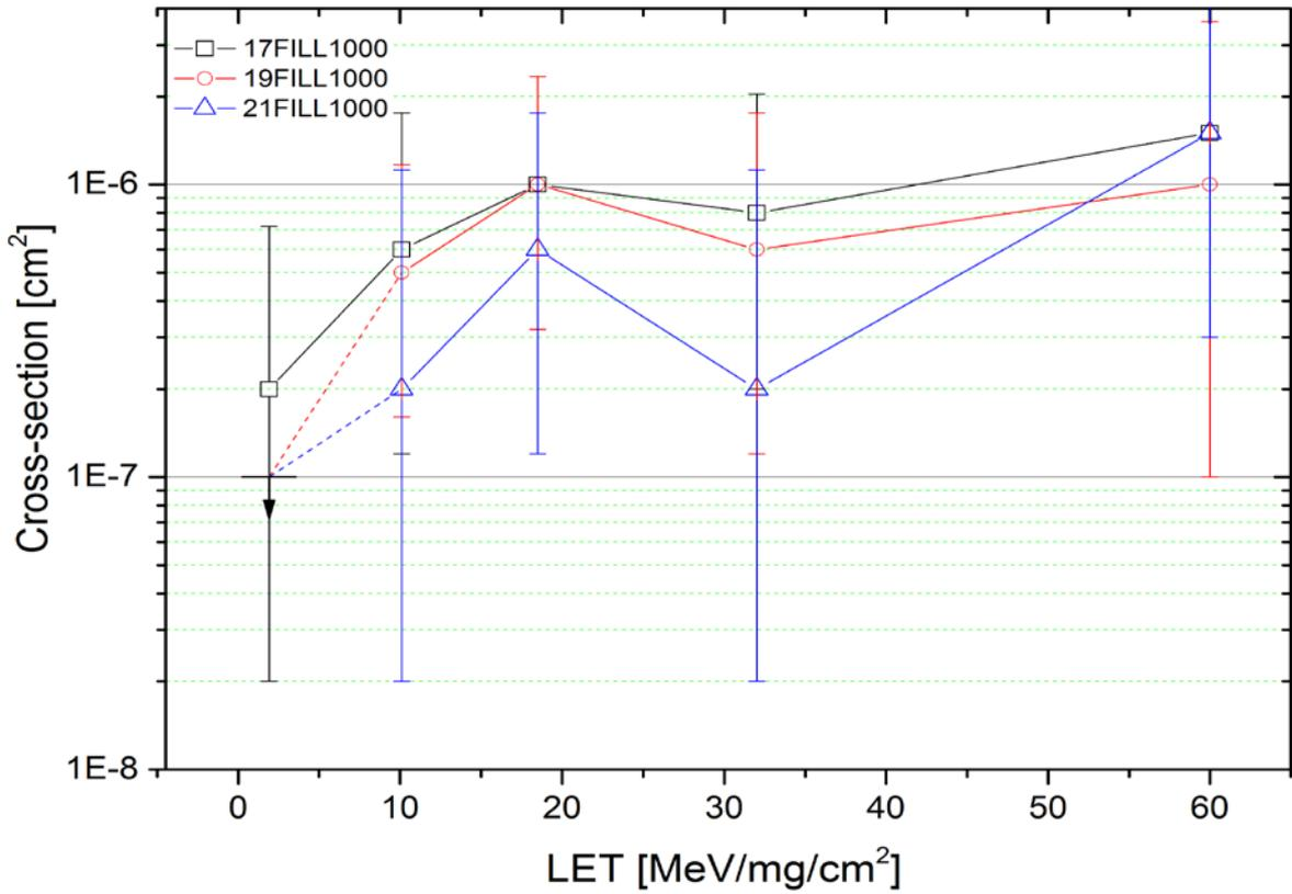
Figure 3-41 "FILL" cross-section for Vitesse components at 1000 Mb/s mode (heat off).
