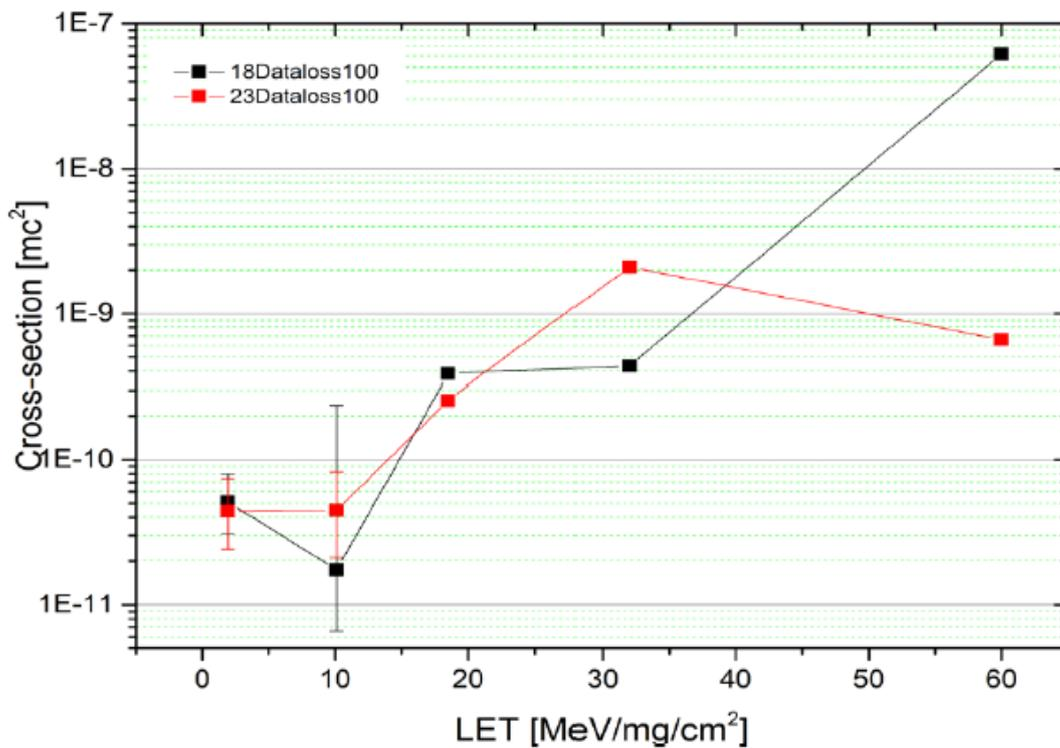
Figure 3-26 Data loss cross-section for Marvell components at 100 Mb/s mode (heat off).
