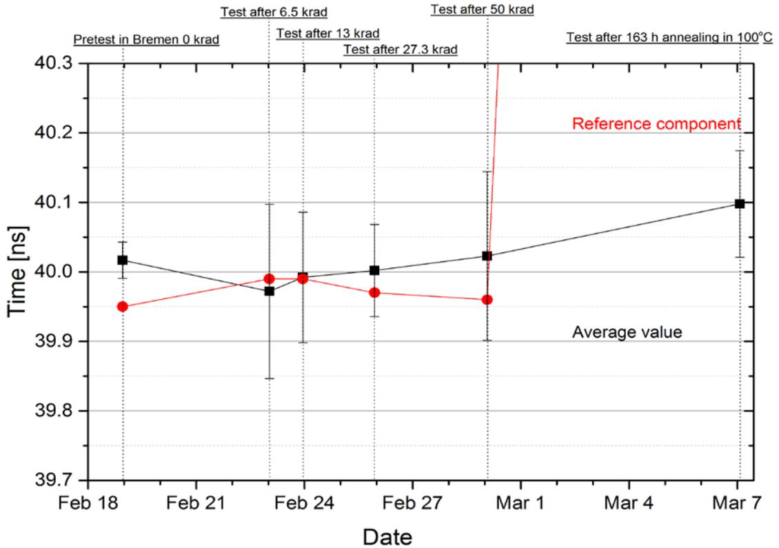
Figure 3-14 Average of RX Clock to Data delay for Vitesse at 100Mbps compared with reference component.
