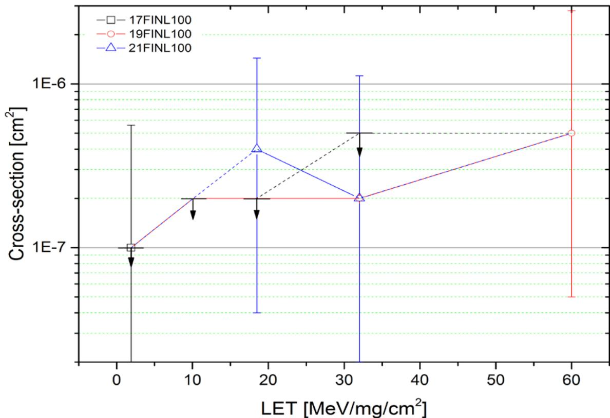
Figure 3-38 "FINL" cross-section for Vitesse components at 100 Mb/s mode (heat off).
