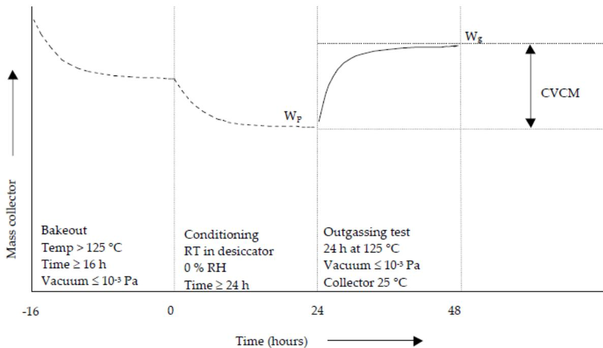
Figure 4-7 Overview of the collector plate parameters
