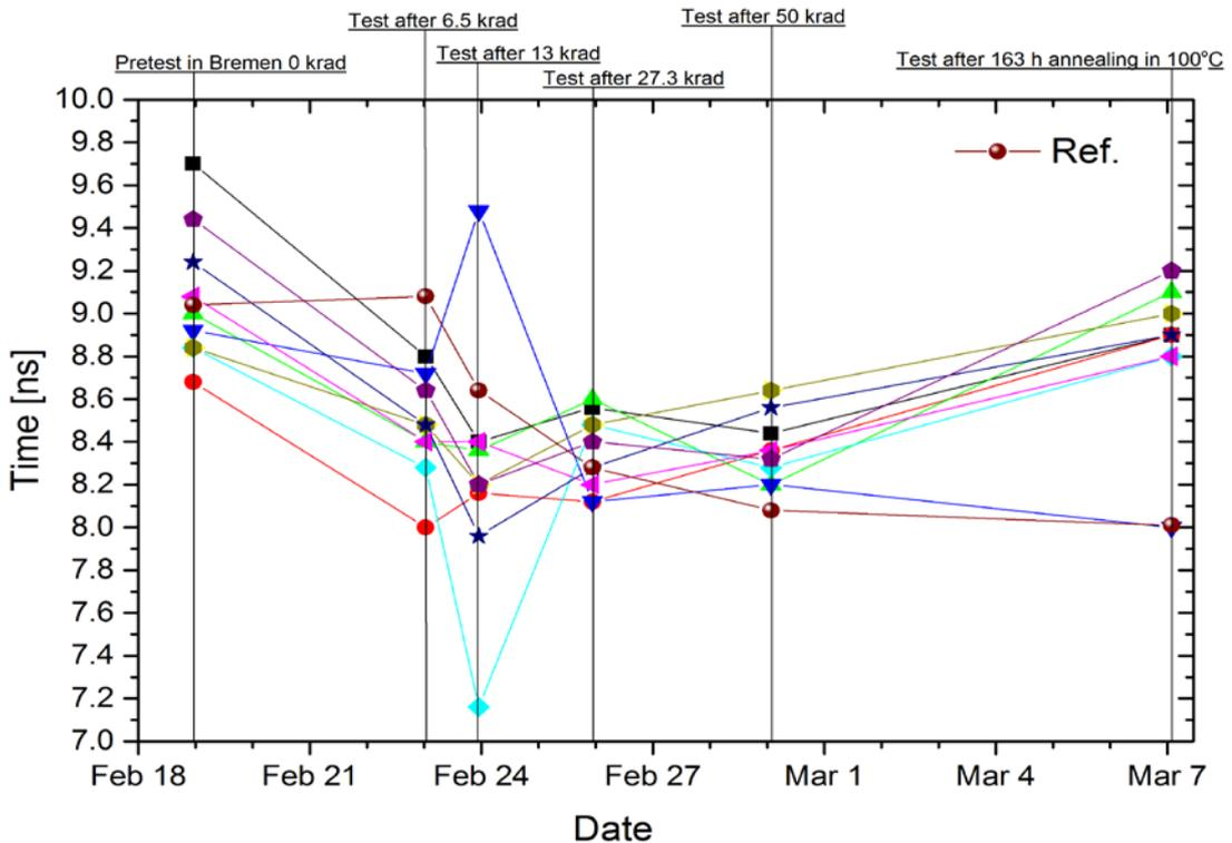
Figure 3-15 RX Clock to Data delay for Vitesse 100MB/s.
