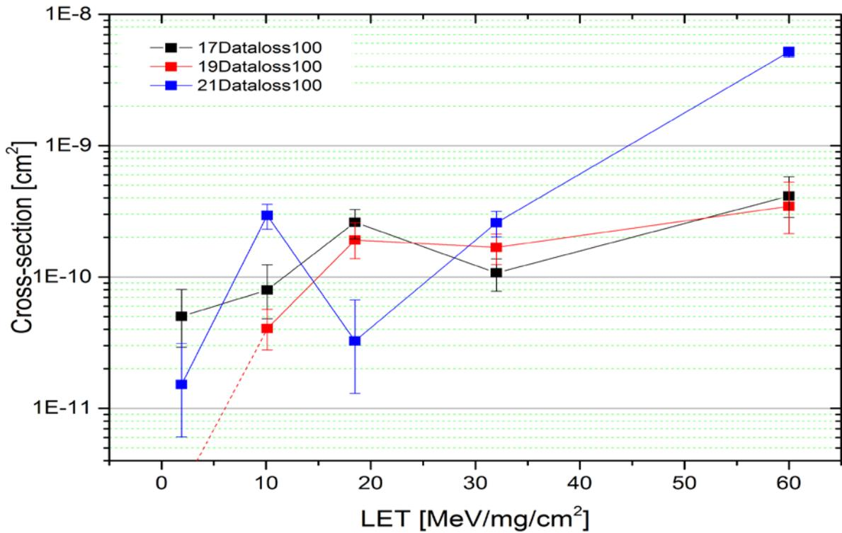
Figure 3-35 "Data loss" cross-section for Vitesse components at 100Mb/s mode (heat off).
