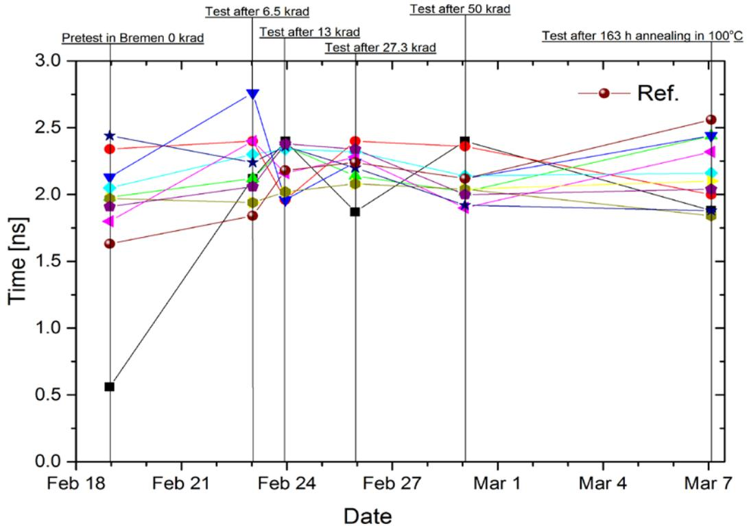
Figure 3-19 RX Clock to Data delay for Vitesse 1000MB/s.
