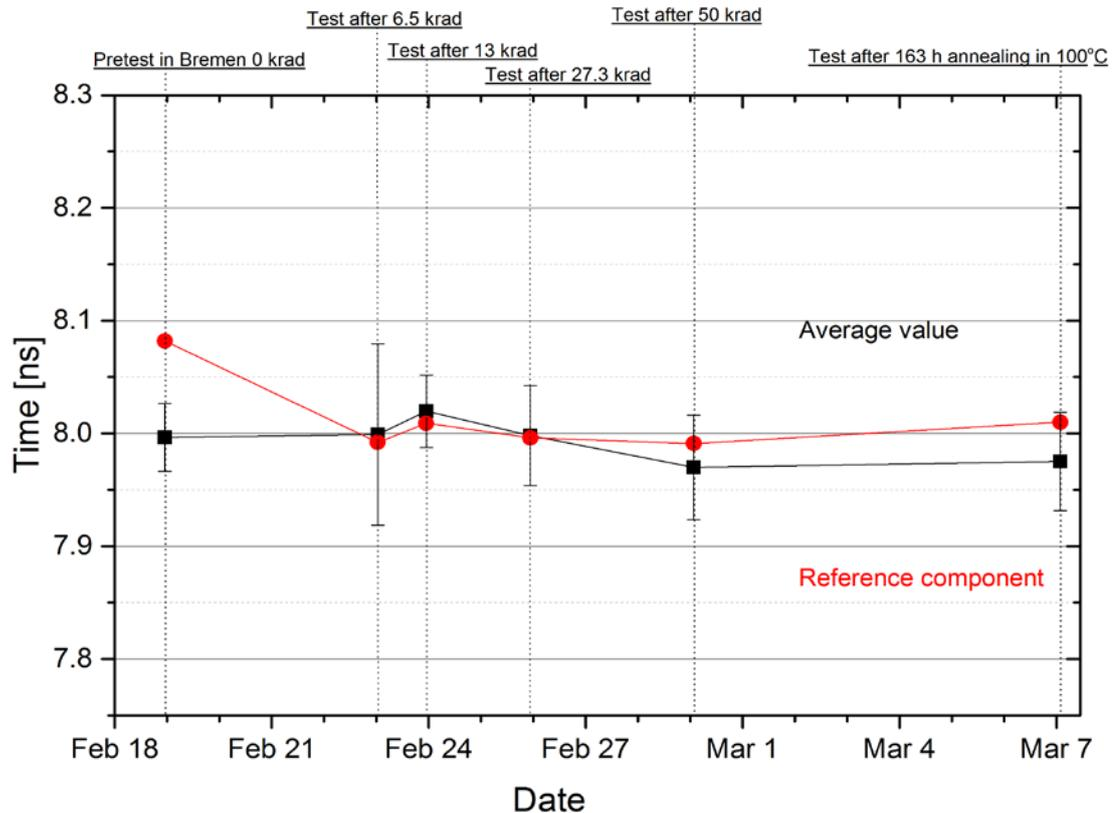
Figure 3-18 Average of RX Clock period for Vitesse component at 1000Mbps compared with reference component.
