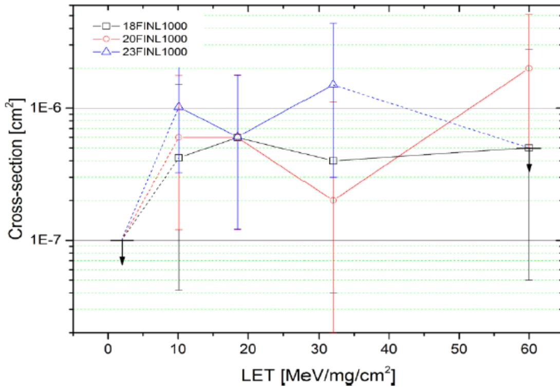
Figure 3-31 Link lost recovery “LLR” cross-section for Marvell components at 1000 Mb/s mode (heat off).
