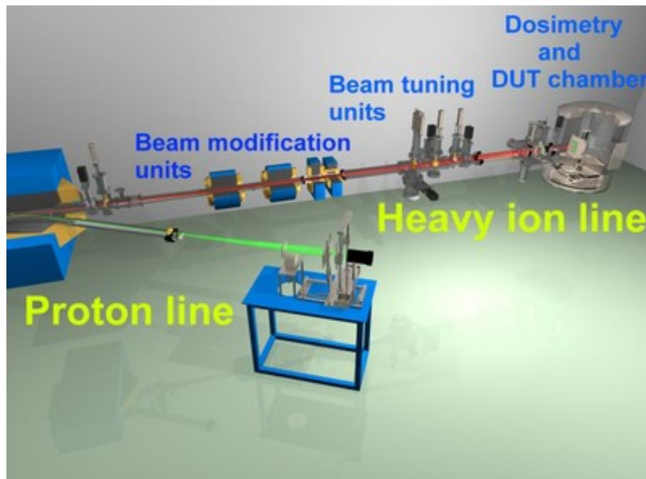
Figure 3-21 Heavy ion and low energy proton beam line with the vacuum chamber at RADEF. High energy protons are taken to air using the beam line at front.
