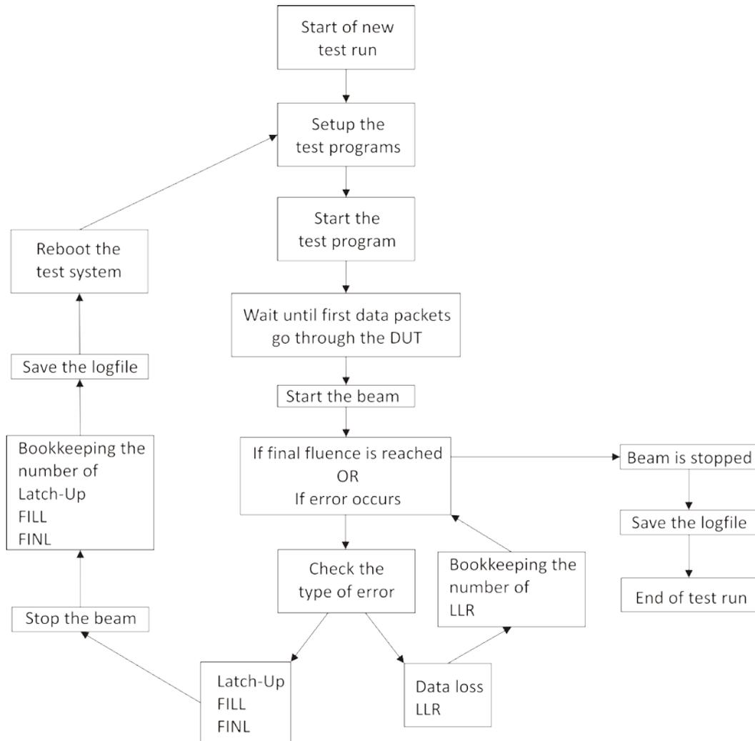
Figure 3-24 Test logic for "Heat off" mode for the SEU events.
