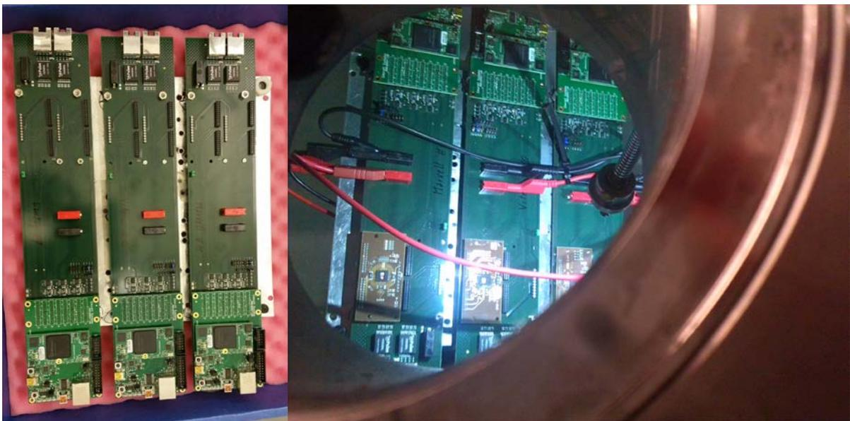
Figure 3-23 Motherboards without the PHYs and with PHYs in the vacuum chamber
