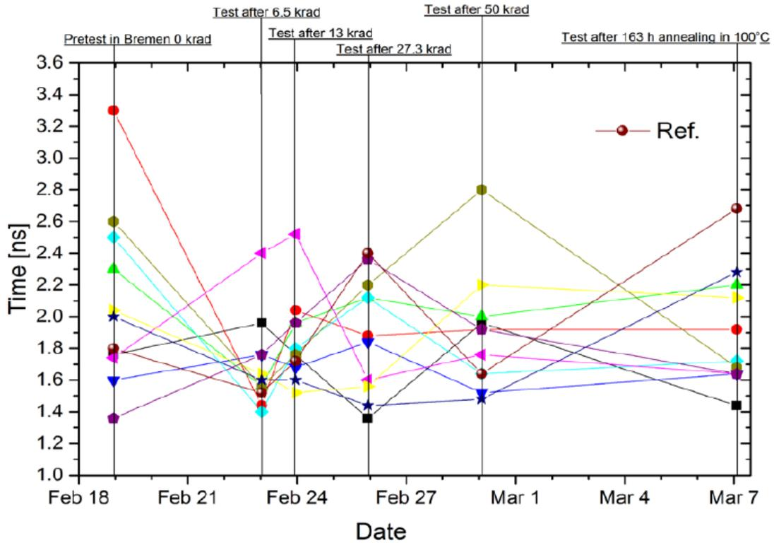
Figure 3-11 RX Clock to Data delay for Marvell 1000MB/s
