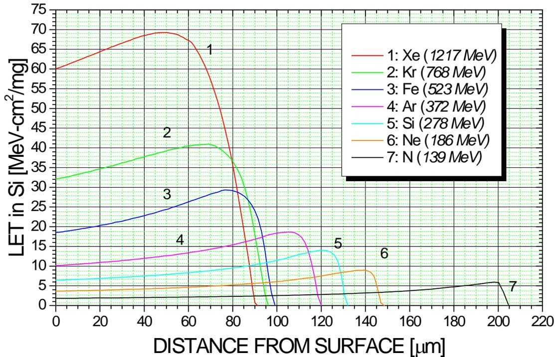
Figure 3-22 LET curves of 9.3 MeV/u cocktail ions in silicon.
