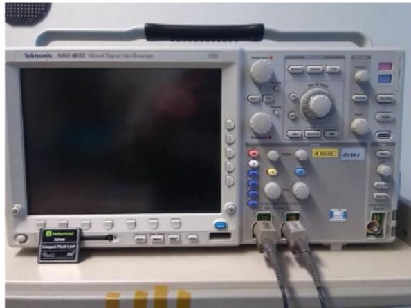
For each PHYDUT, measure RX Clock and Data3 at SF2 STARTERKIT (P12 Pin 3 and 7).
