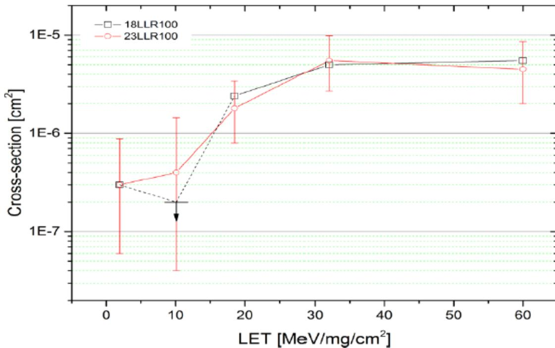
Figure 3-28 Link lost recovery “LLR” cross-section for Marvell components at 100 Mb/s mode (heat off).
