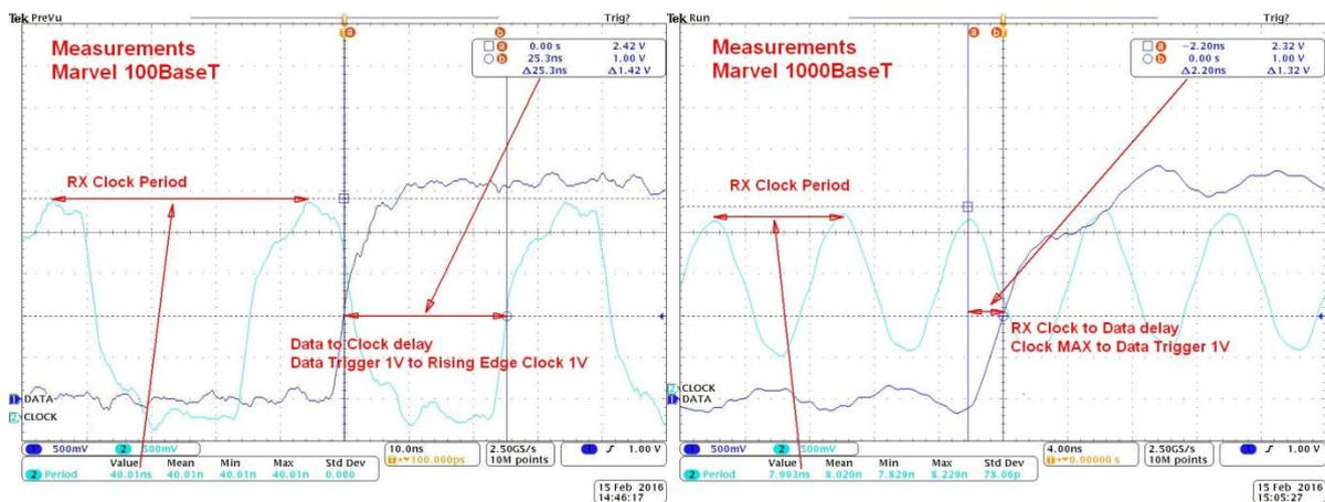
Figure 4-4 Measurements key parameters of test samples, here for Marvell
