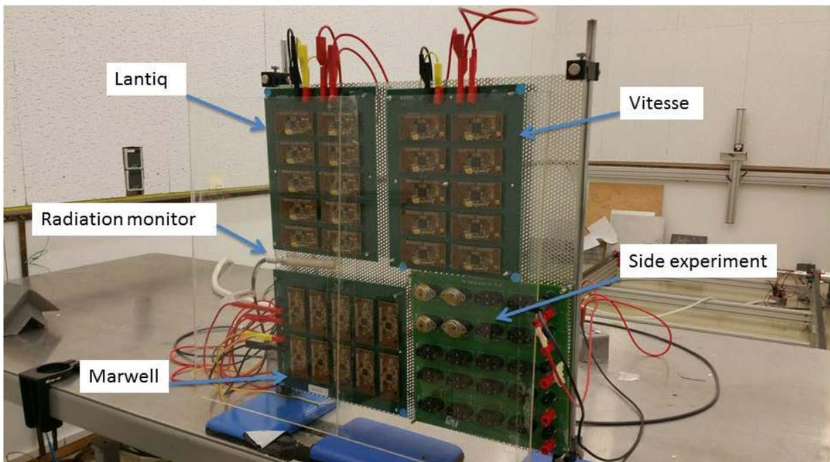
Figure 3-3 Components ready for TID irradiation
