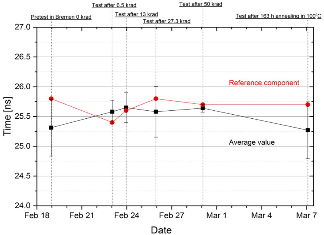
Figure 3-8 Average of RX Clock to Data delay for Marvell at 100MB/s compared with reference component.
