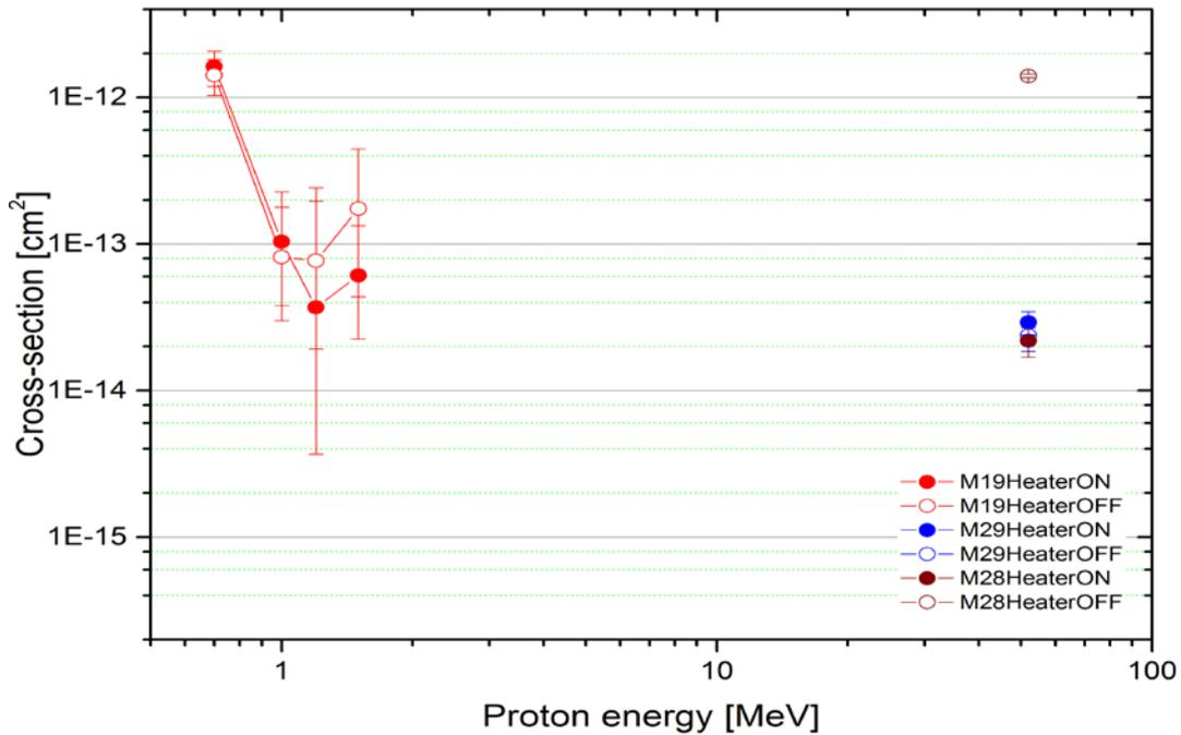
Figure 3-45 "Data loss" cross-sections for Marvell components in proton irradiations. Point for component 28 with heat off differs from the other 52 MeV points two orders of magnitudes. When analyzing the data it was noticed that component has had some problems during last 2 min of the 6 min long irradiation. During that last 2 min it lost half of the data packets. Reason for this is not known.
