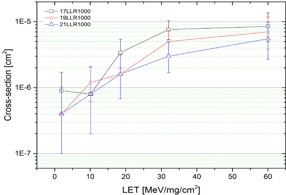
Figure 3-37 "LLR" cross-section for Vitesse components at 1000 Mb/s mode (heat off).
