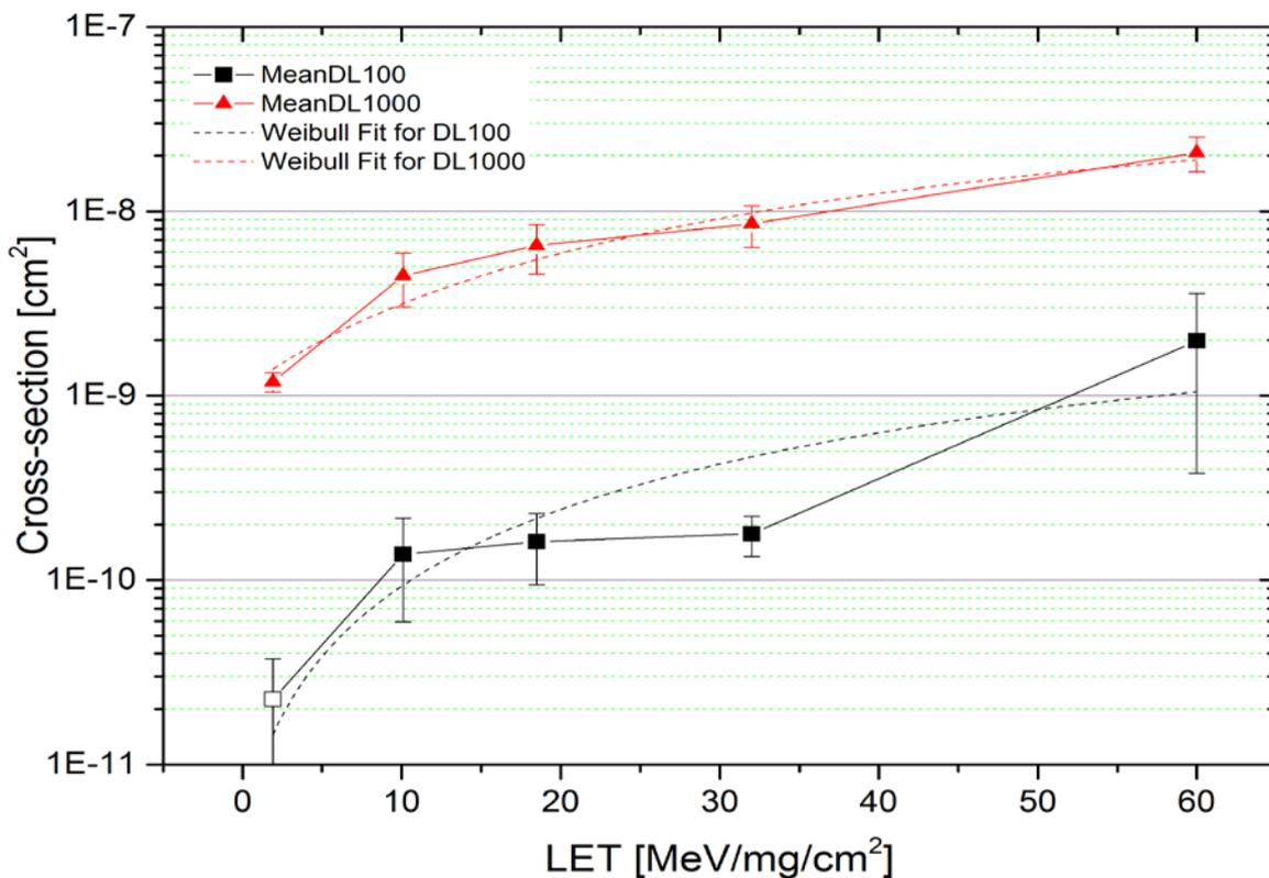
Figure 3-44 Mean value of "Data loss" cross-section as a function of LET for Vitesse components (heat off).
