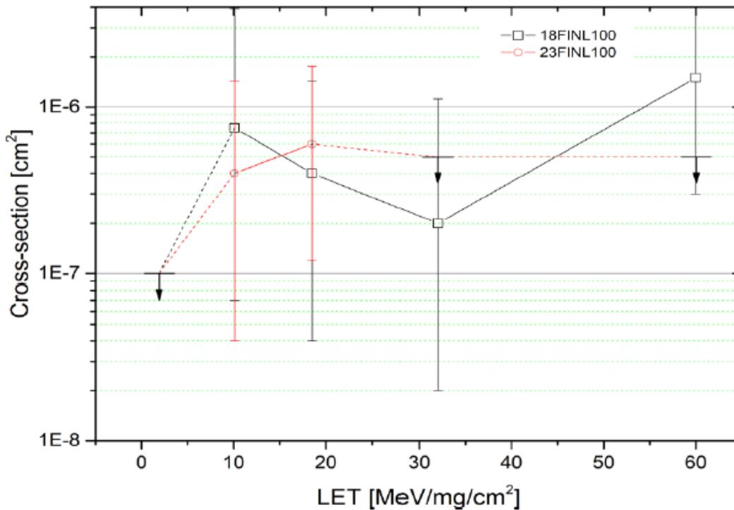
Figure 3-30 “FINL” cross-section for Marvell components at 100 Mb/s mode (heat off).
