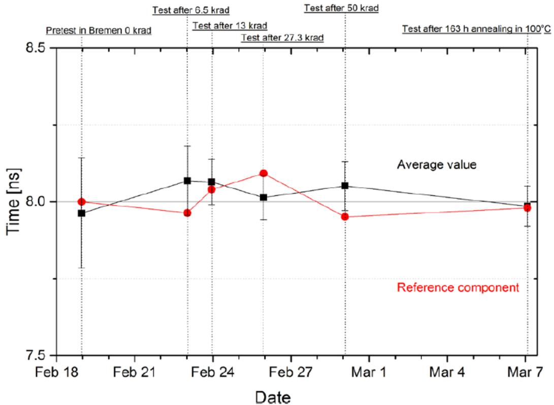
Figure 3-10 Average of RX Clock period for Marvell at 1000MB/s compared with reference component.
