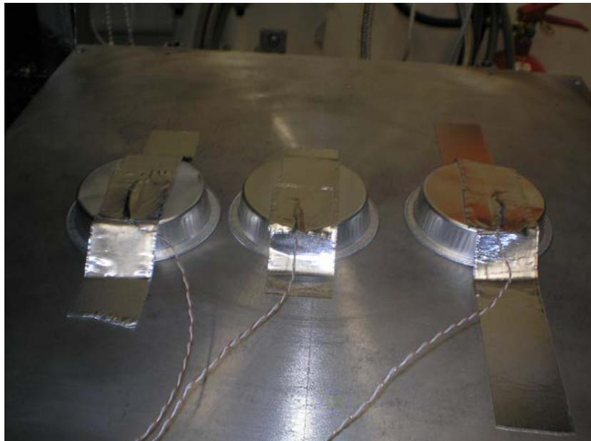
The devices under test were placed and fixed in a vacuum chamber. The temperature was checked by using three thermocouples of Type I IEC 584-3mod DIN 43722.
