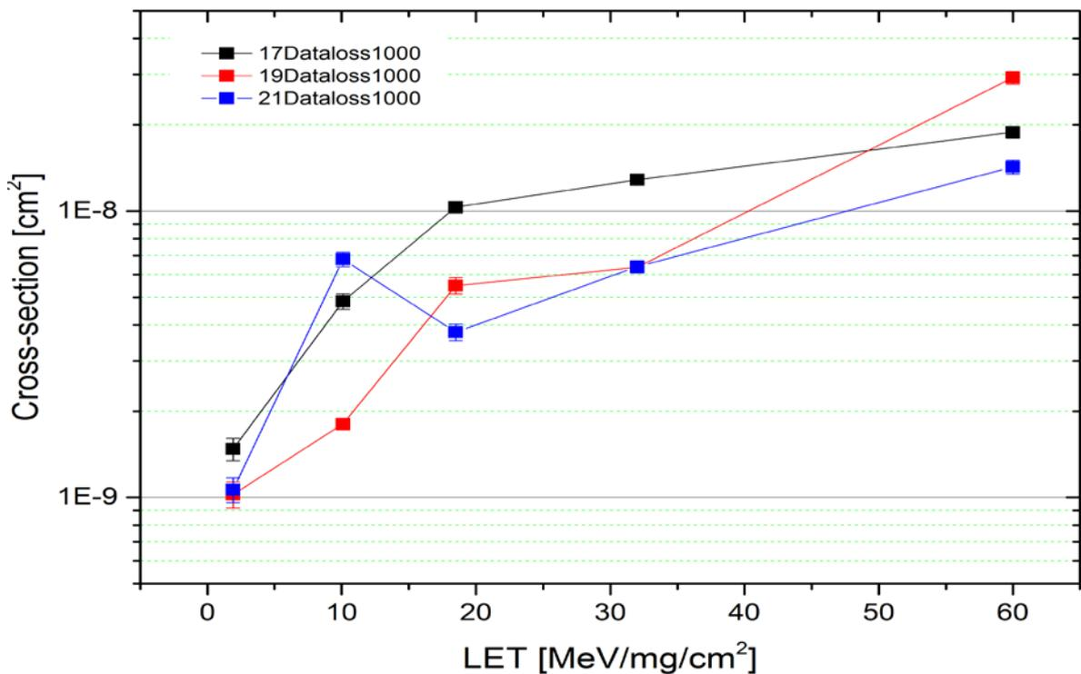
Figure 3-36 "LLR" cross-section for Vitesse components at 100 Mb/s mode (heat off).
