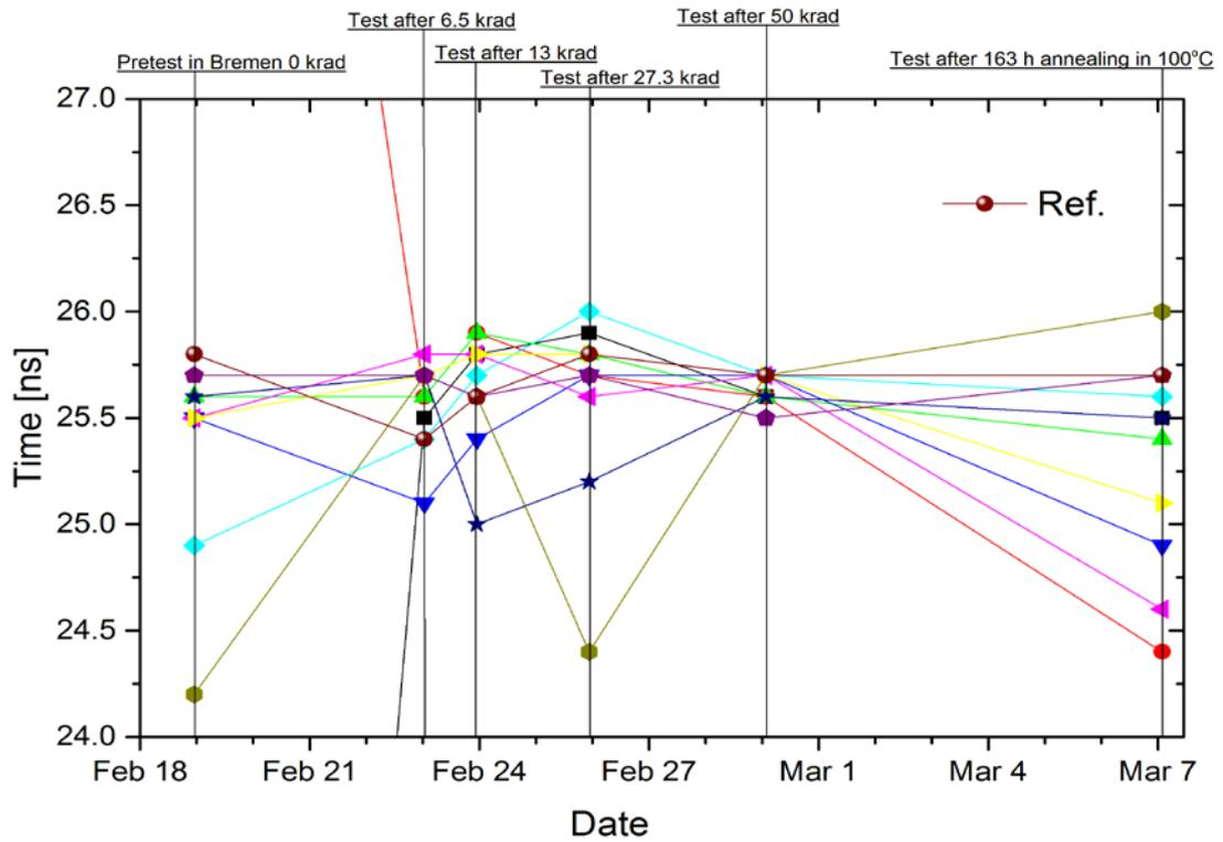
Figure 3-7 RX Clock to Data delay for Marvell 100MBps.
