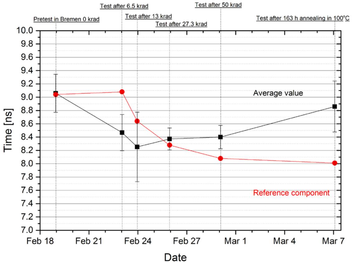
Figure 3-16 Average of RX Clock to Data delay for Vitesse at 100Mbps compared with reference component.
