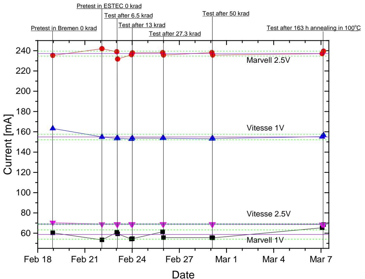
Figure 3-4 Evolution of current consumption of 10 Marvell and 10 Vitesse components over irradiation and annealing. Violet lines are average values and green dashed lines are average value ± standard deviation.
