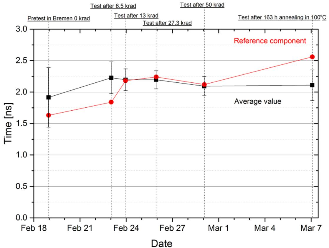
Figure 3-20 Average of RX Clock to Data delay for Vitesse at 1000MB/s compared with reference component.
