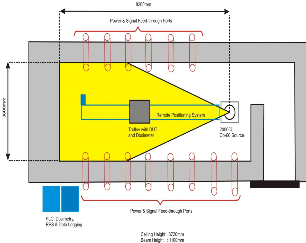
Figure 3-2 Layout of ESA-ESTEC Co-60 Facility in Noordwijk
