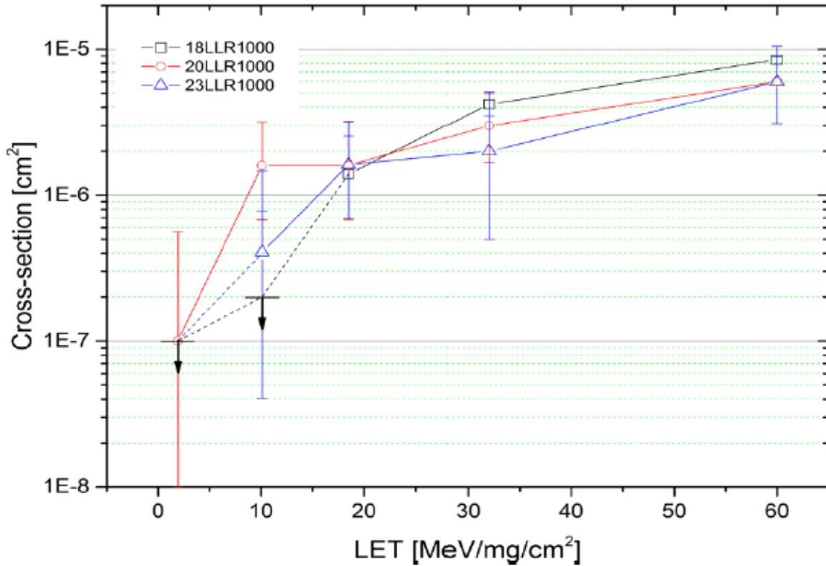
Figure 3-29 Link lost recovery “LLR” cross-section for Marvell components at 1000 Mb/s mode (heat off).
