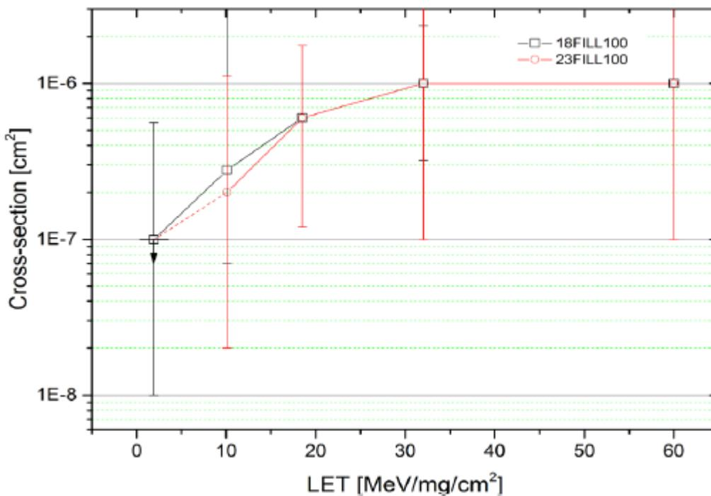
Figure 3-32 FILL cross.section for Marvell at 100MB/s heat off.
