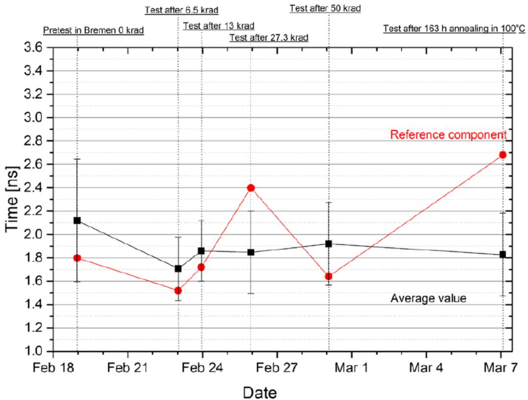
Figure 3-12 Average of RX Clock to Data delay for tested Marvell at 1000MB/s compared with reference component.
