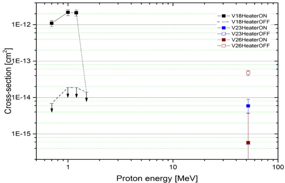
Figure 3-46 "Data loss" cross-sections for Vitesse components in proton irradiations.
