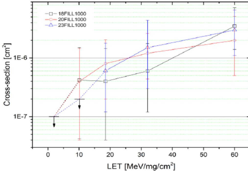
Figure 3-33 FILL cross-section for Marvell at 1Gb/s mode heat off.
