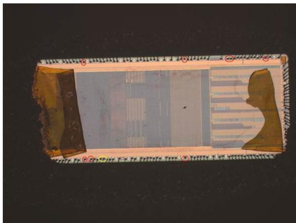
A number of broken contacts can be seen indicated in red in the picture. Two possible explanations could be found:
