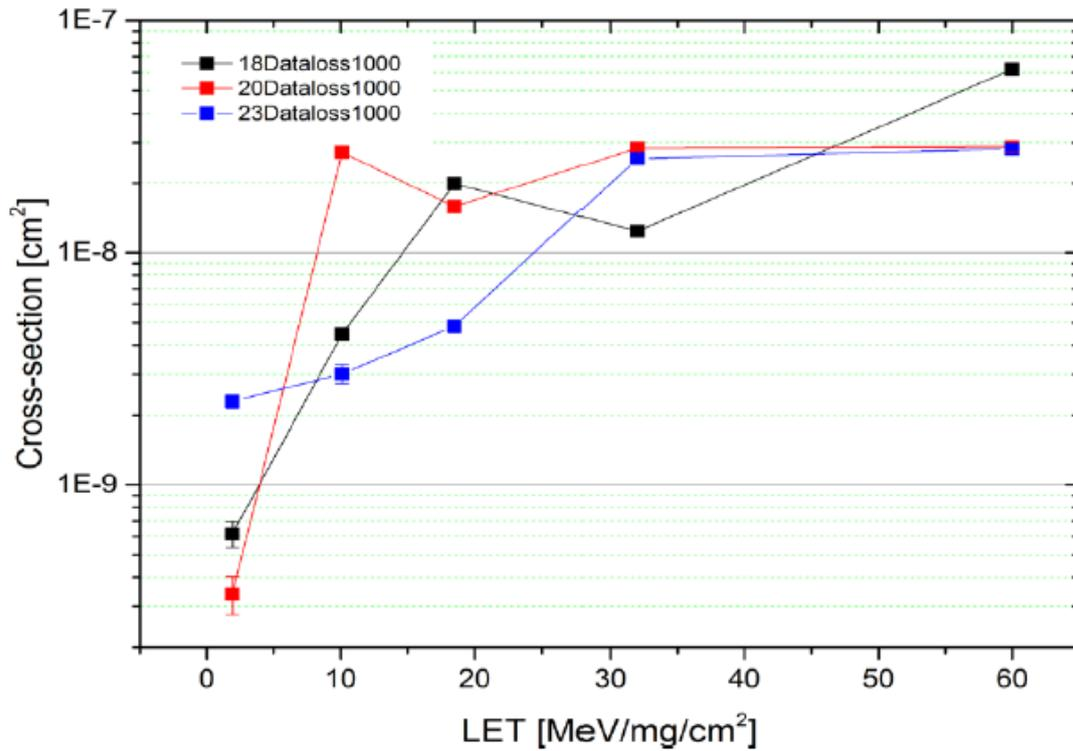
Figure 3-27 Data loss cross-section for Marvell components at 1000 Mb/s mode (heat off).
