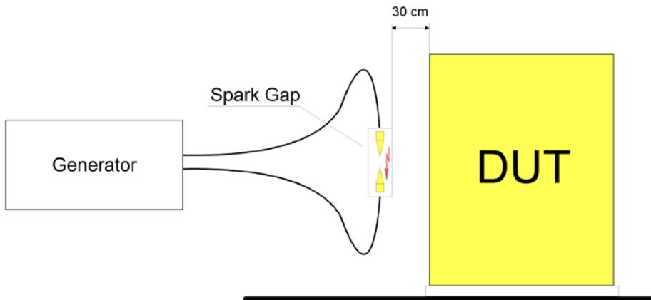
Figure 4-1 Test Setup for radiated arc discharge susceptibility.
