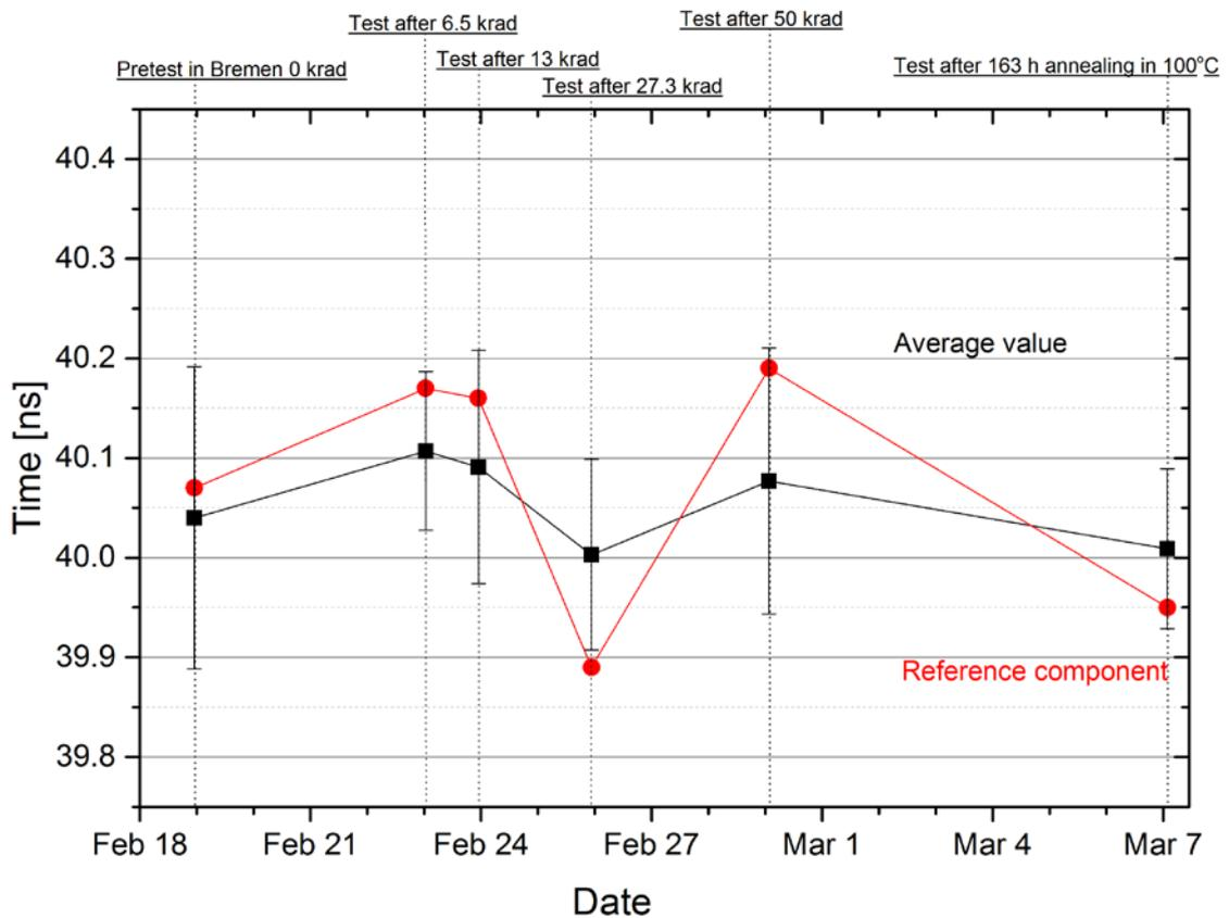
Figure 3-6 Average of RX Clock period for Marvell at 100MB/s compared with reference component.
