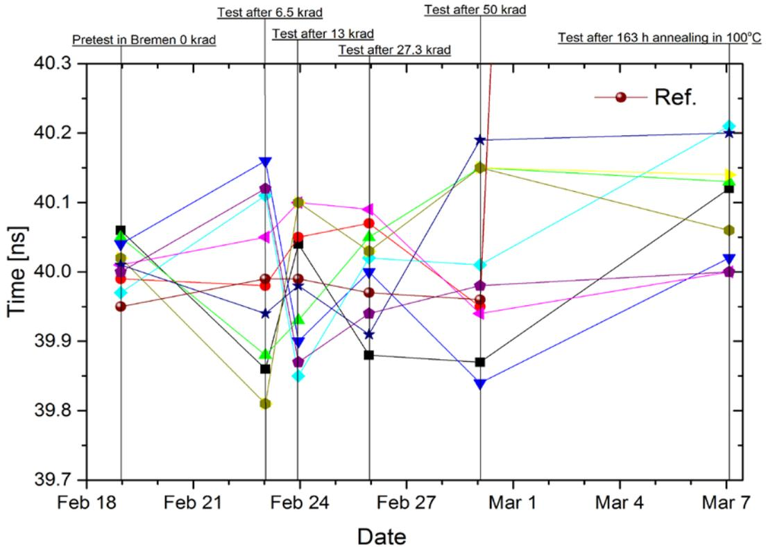
Figure 3-13 RX Clock period for Vitesse 100MB/s.
