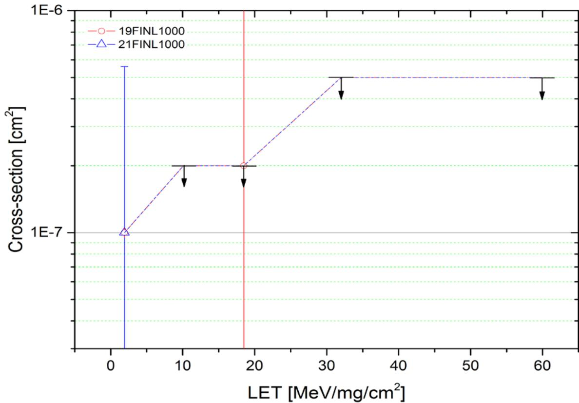
Figure 3-39 "FINL" cross-section for Vitesse components at 1000 Mb/s mode (heat off).
