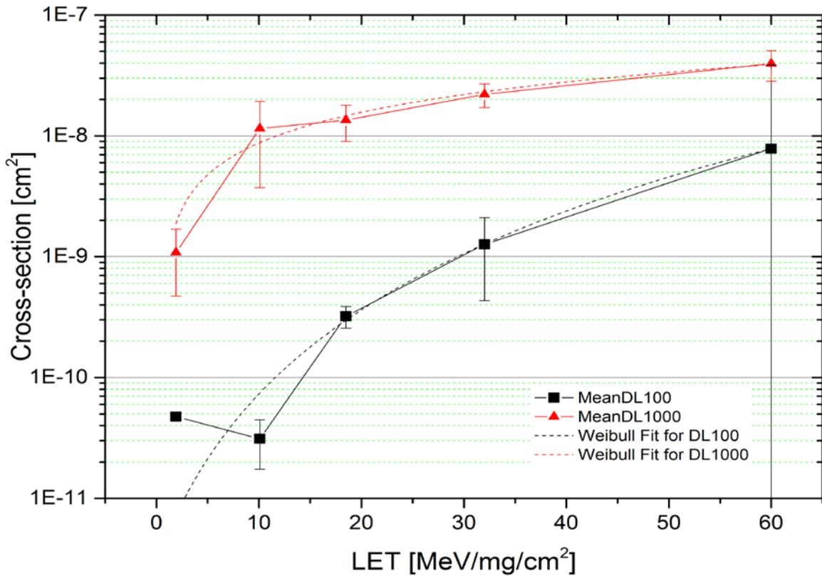
Figure 3-43 Mean value of "Data loss" cross-section as a function of LET for Marvell components (heat off).
