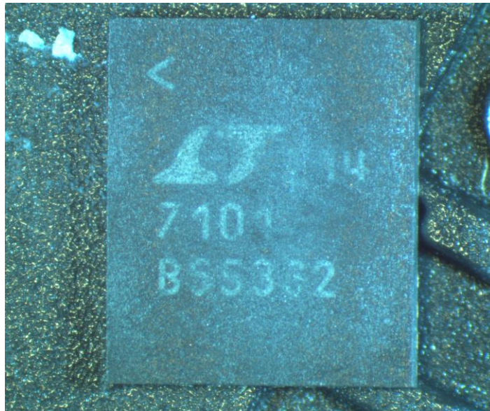
Figure 3: Microscope Picture of the package marking of the LT7101
