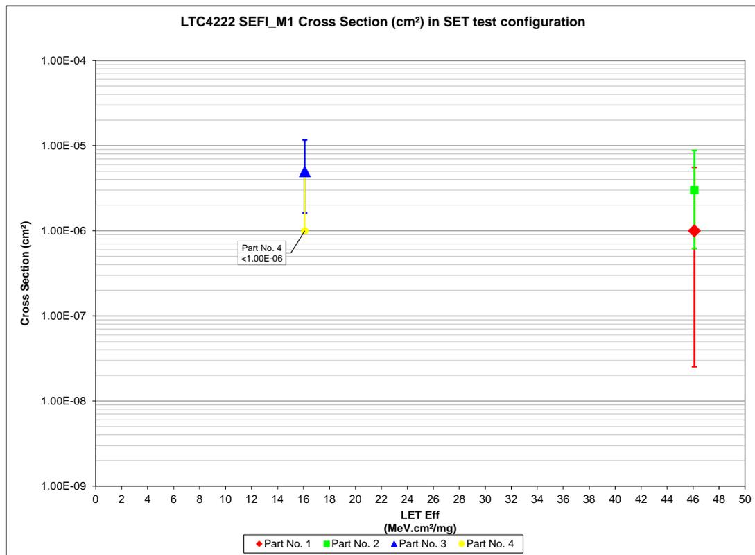
Figure 15: LTC4222CG SEFI\_M1 cross section curve in SET test configuration
