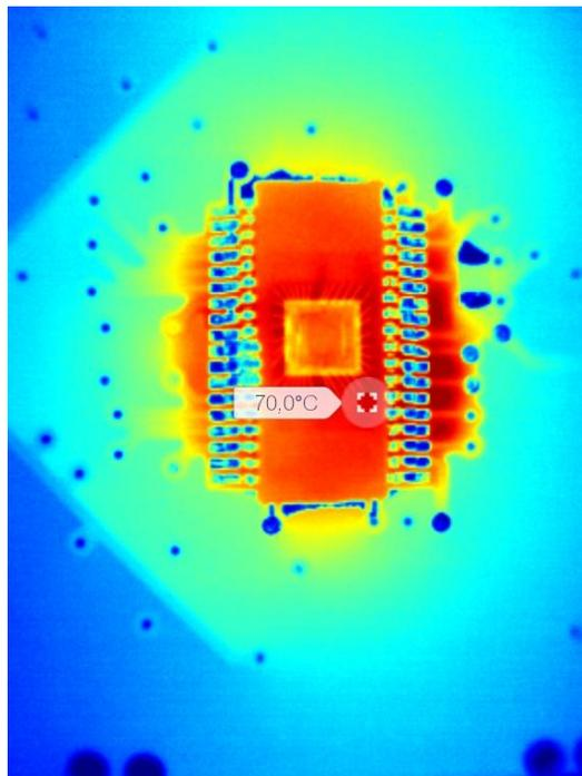
Figure 9: Thermal image of LTC4222CG heated to  $70^\circ\text{C}$
