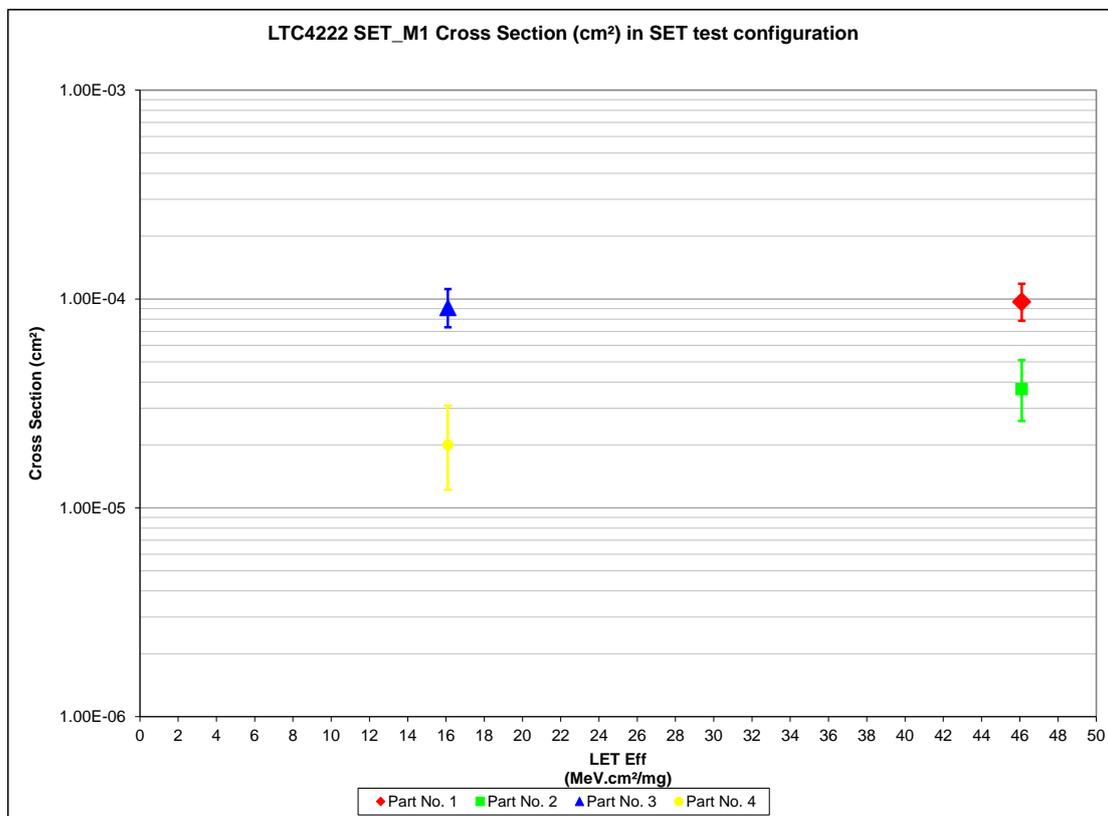
Figure 11: LTC4222CG SET\_M1 cross section curve in SET test configuration
