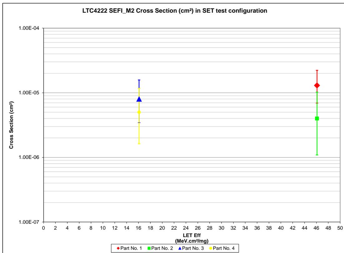
Figure 16: LTC4222CG SEFI\_M2 cross section curve in SET test configuration
