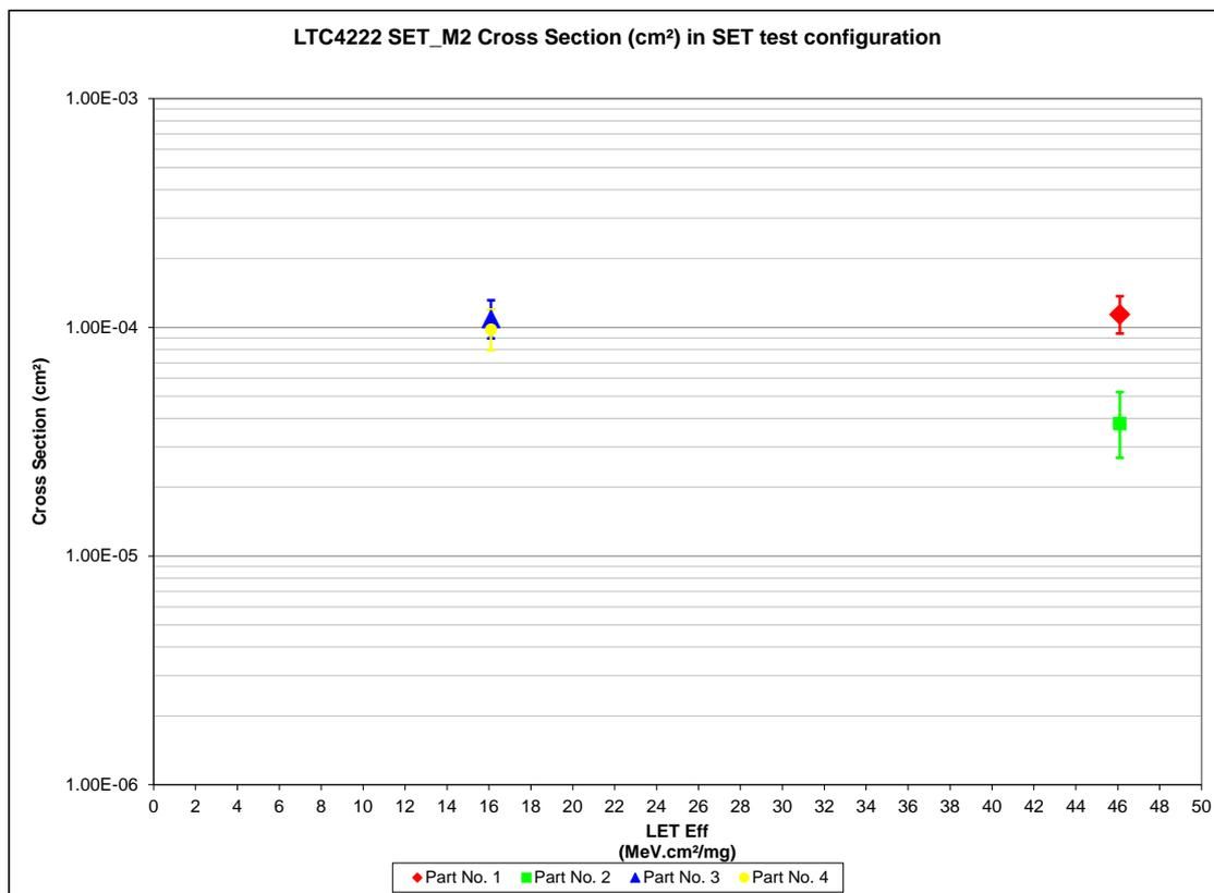
Figure 13: LTC4222CG SET\_M2 cross section curve in SET test configuration
