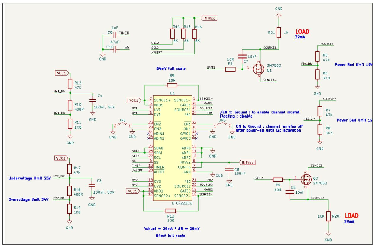
**Figure 10: Test board schematic**
