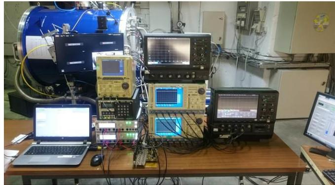
Figure 4: Typical UCL HIF test bench setup
