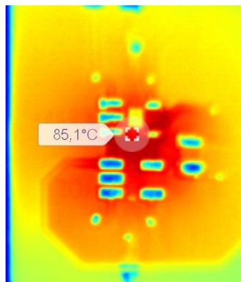
Figure 9: Thermal image of TPS3820-33DBV heated to  $85^\circ\text{C}$
