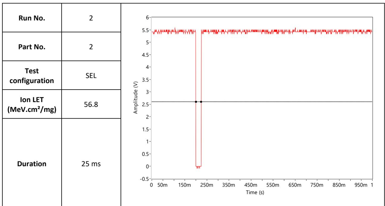
Figure 16: SET /RESET shortest case duration
