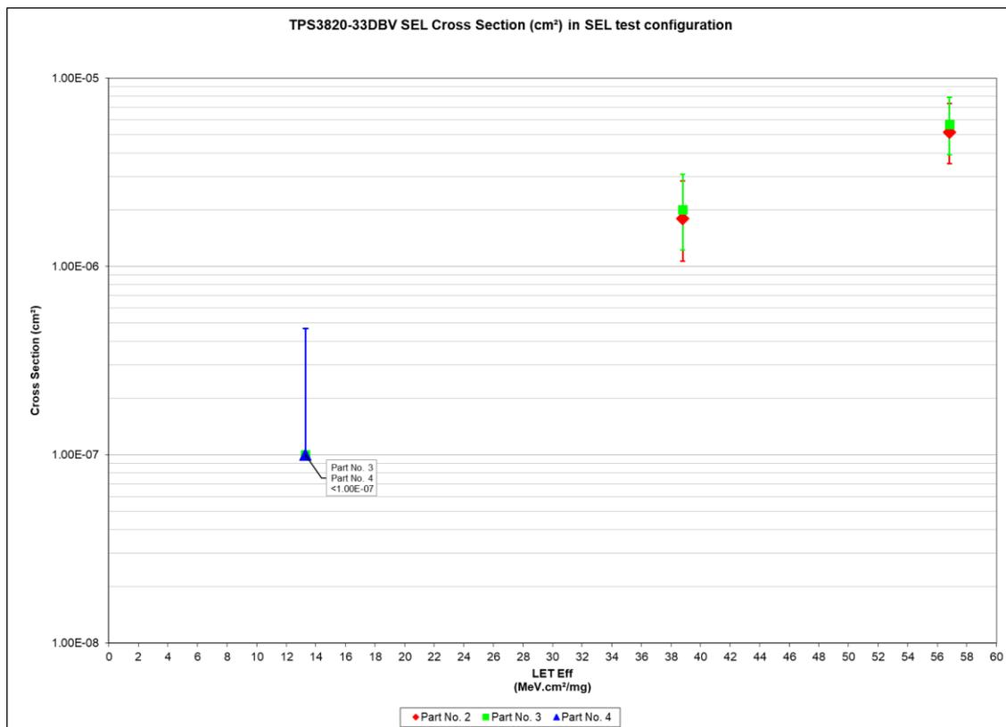
**Figure 11: TPS3820-33DBV SEL cross section curve in SEL test configuration**
