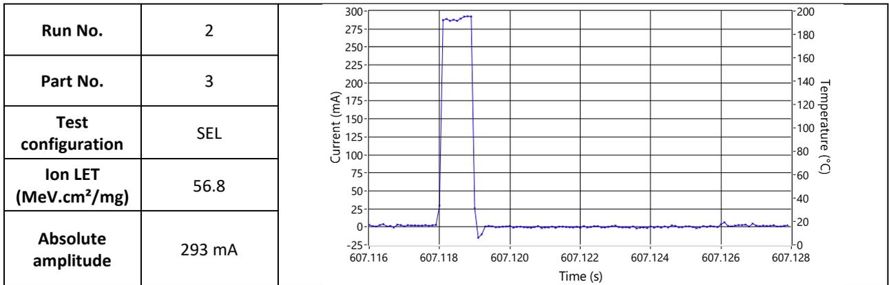
**Figure 13: SEL smallest case amplitude**
