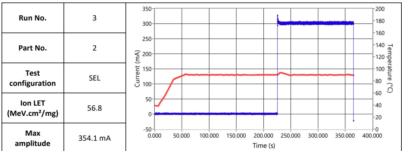
**Figure 14: Unprotected run**
