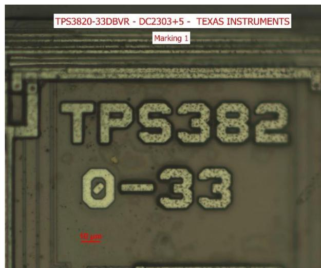
Figure 3: Picture of the die markings
