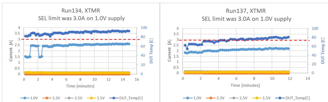
However, it had no impact of the number of errors recorded. E.g the recorded error cross section for fails of the CPU was 2.6e-3 cm<sup>2</sup>/device and 2.9e-3 cm<sup>2</sup>/device for run#134 and run#137, respectively. The LET was 10 MeV-cm<sup>2</sup>/mg in these runs. These error rates are much higher than it can expected for an XTMR design.
