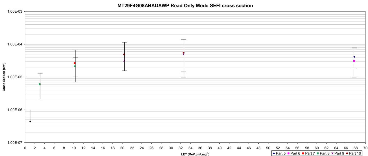
Figure 15: Read Only Mode SEFI cross section curve for MT29F4G08ABADAWP
