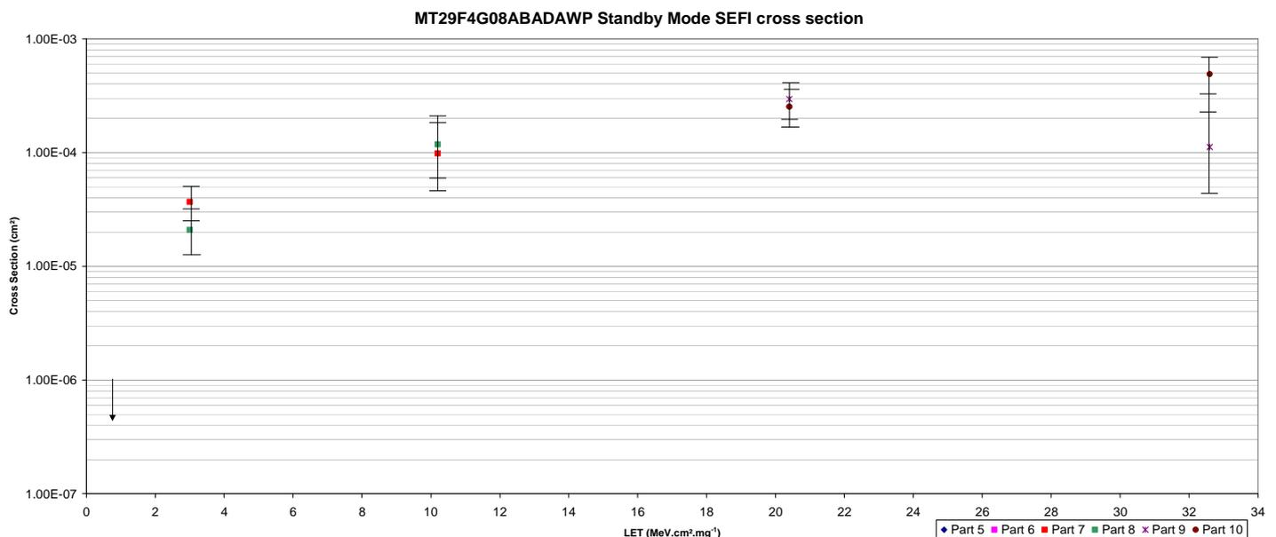
Figure 13: Standby Mode SEFI cross section curve for MT29F4G08ABADAWP
