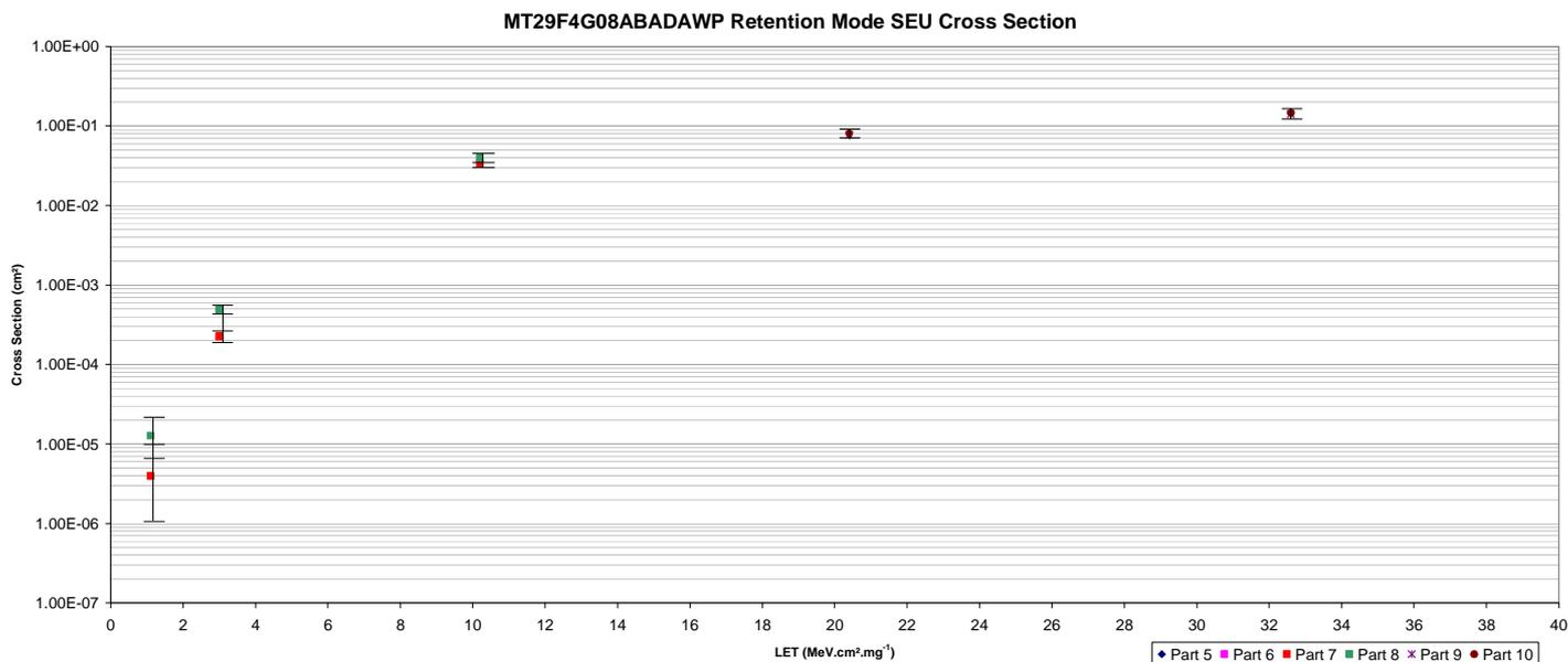
Figure 11: Retention Mode SEU cross section curve for MT29F4G08ABADAWP
