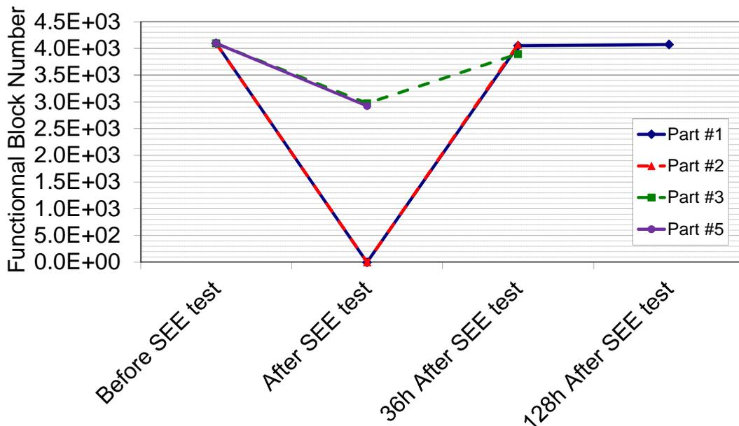
Figure 7 : MT29F4G08AAC Number of functional blocks before and after SEE test using the Xenon ion
