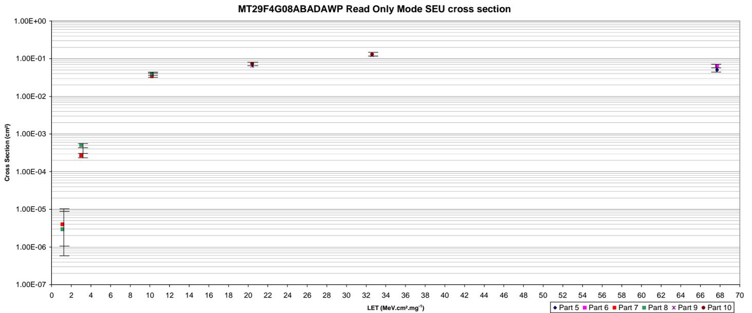
Figure 14: Read Only Mode SEU cross section curve for MT29F4G08ABADAWP
