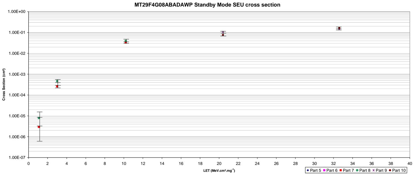
**Figure 12: Standby Mode SEU cross section curve for MT29F4G08ABADAWP**
