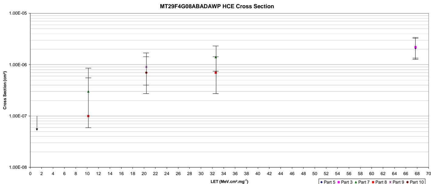
Figure 10: HCE cross section curve for MT29F4G08ABADAWP
