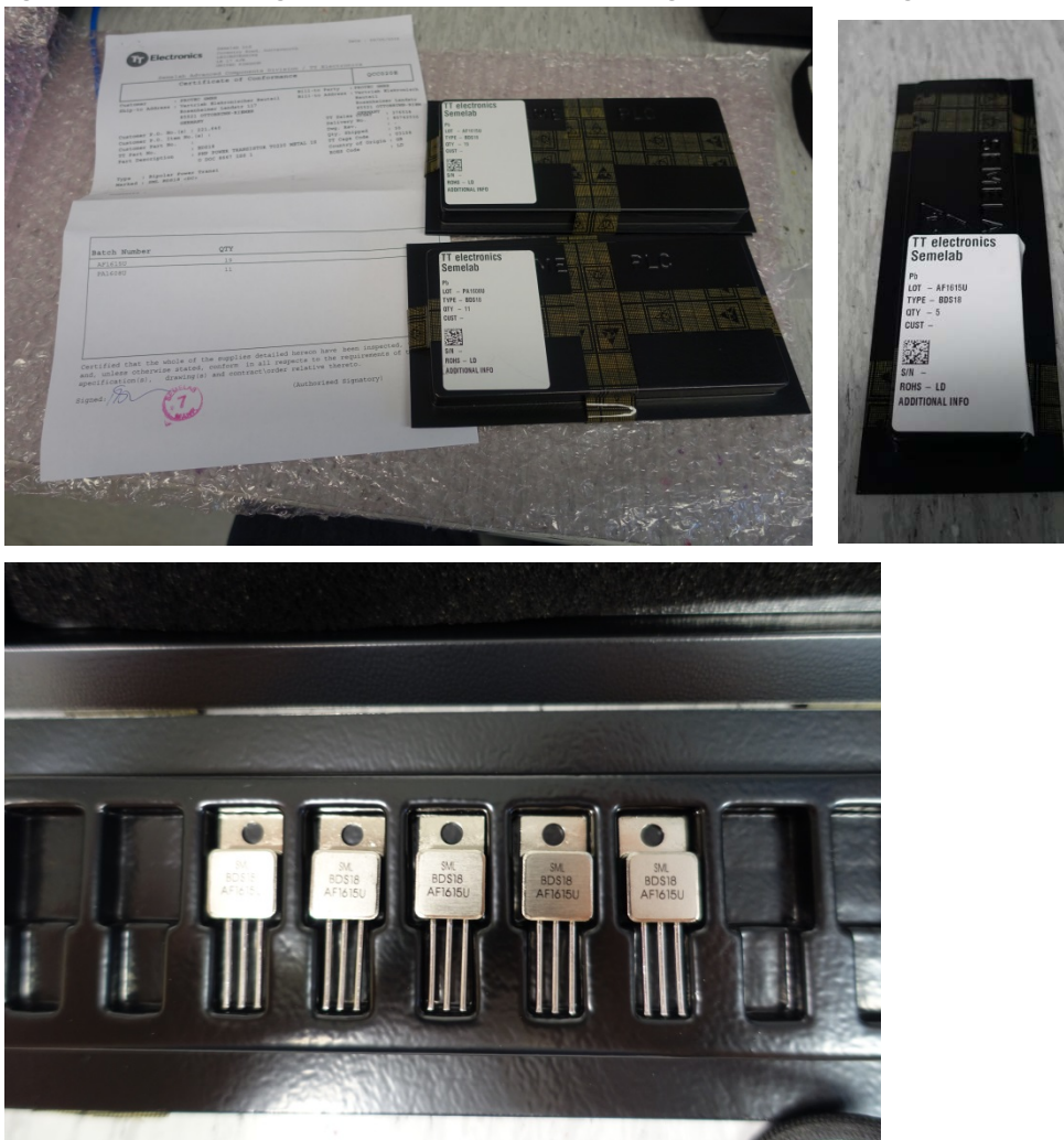
Figure 3: The ESD package with the samples (left: first charge from 2 batches, right and bottom: second procurement)
