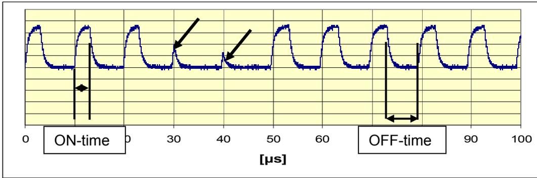
*Fig. 5.1.1 Oscilloscope graph from the output of the UC2845 showing the principal for calculating the length of the too long OFF-time.*
