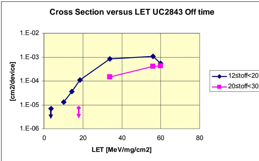
Fig 5.3.3 Too long OFF time cross sections as a function of LET for UC2843.
