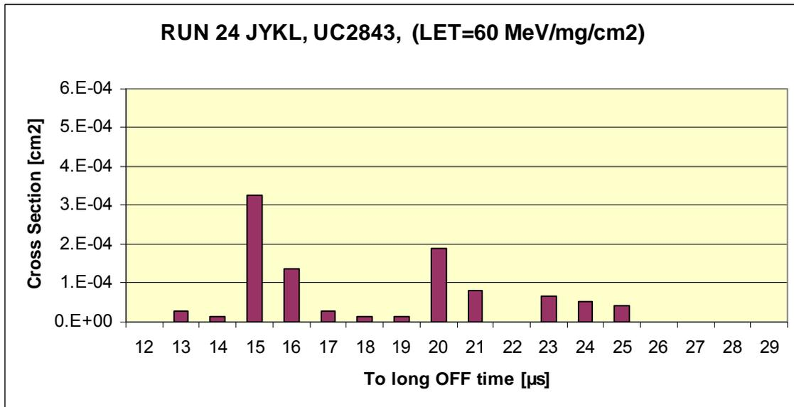
Fig 5.4.9 UC2843 histogram of too long OFF time as a function of the cross section. Irradiation in JYKL with  $^{131}\text{Xe}$  at  $0^\circ$  (LET=60 MeV/mg/cm2).
