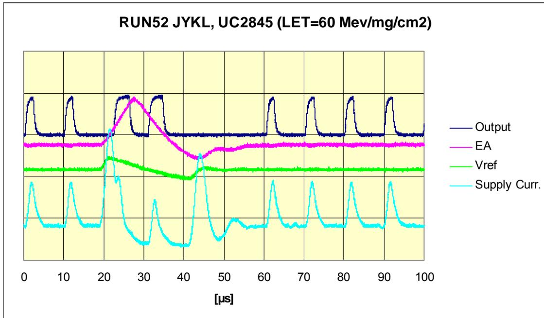
*Fig 5.2.13 Oscilloscope picture of SET in UC2845 triggered by Output with 20V supply voltage.*
