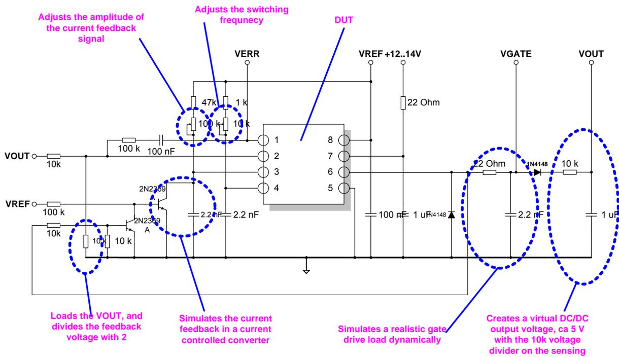
Fig 4.1 Basic Schematic drawing of the biasing of the PWM, the drawing is taken from ref [3]
