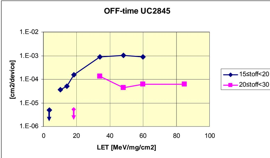
Fig 5.3.1 Too long OFF time cross sections as a function of LET for UC2845.
