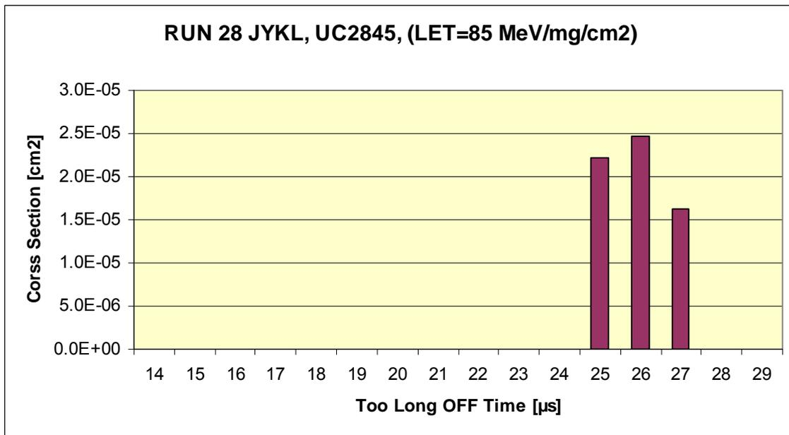
Fig 5.4.12 UC2845 histogram of too long OFF time as a function of the cross section with oscilloscope trigger conditions >22µs. The test was performed to collect better statistics on the longer OFF times. Irradiation in JYKL with <sup>131</sup>Xe at 45° (LET=85 MeV/mg/cm2).
