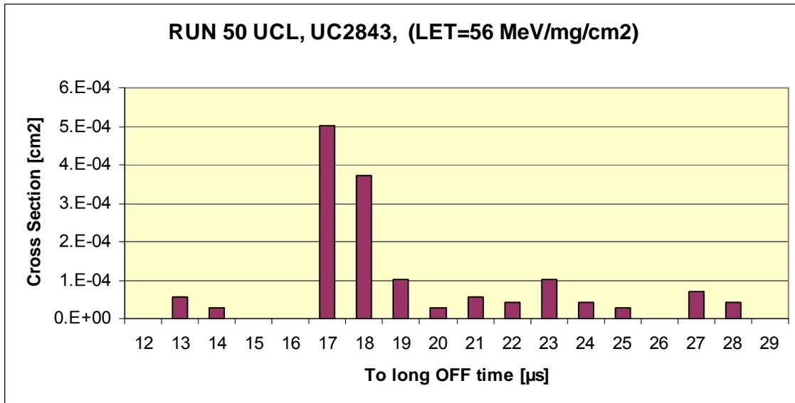
Fig 5.4.8 UC2843 histogram of too long OFF time as a function of the cross section. Irradiation at UCL with  $^{131}\text{Xe}$  at  $0^\circ$  (LET=56 MeV/mg/cm2).
