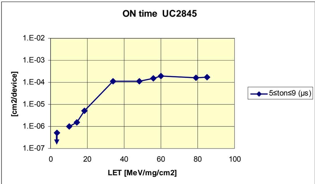
Fig 5.3.2 Too long ON time cross sections as a function of LET for UC2845.
