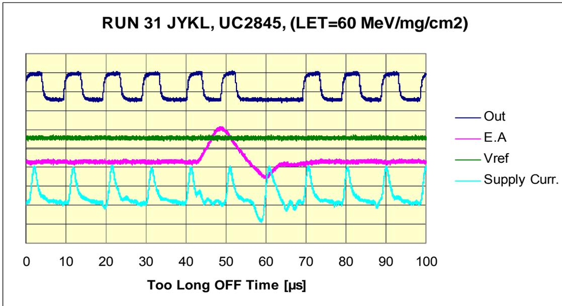
Fig 5.2.3 UC2845. Too long OFF time triggered by Output with EA effected
