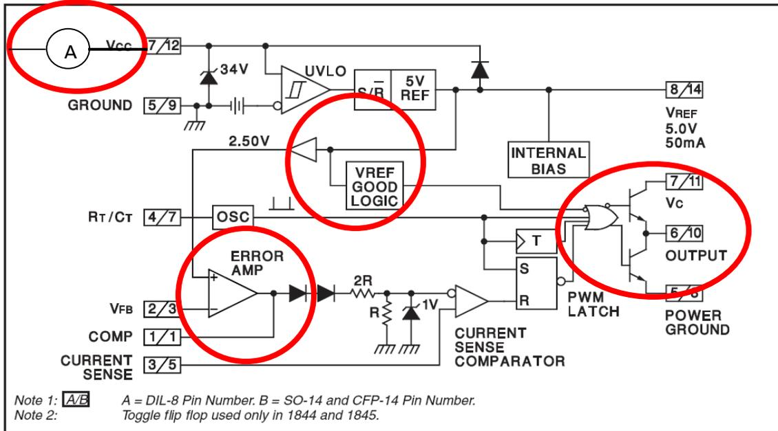
Fig 5.2.1 Block diagram of UC2845. The different functions monitored during irradiations are marked with red circles.
