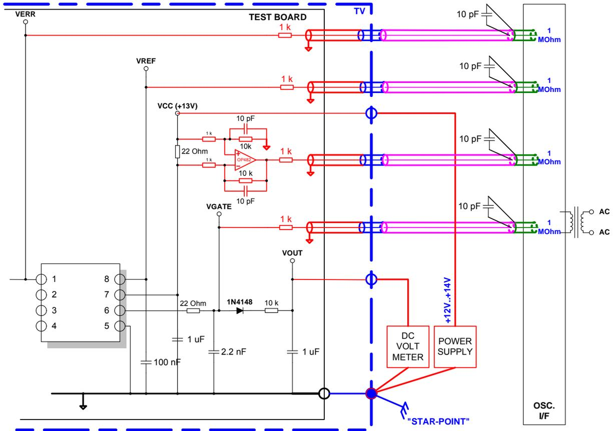
Fig 4.2 Test interface and grounding diagram used for the irradiation tests. The drawing is taken from ref [3].
