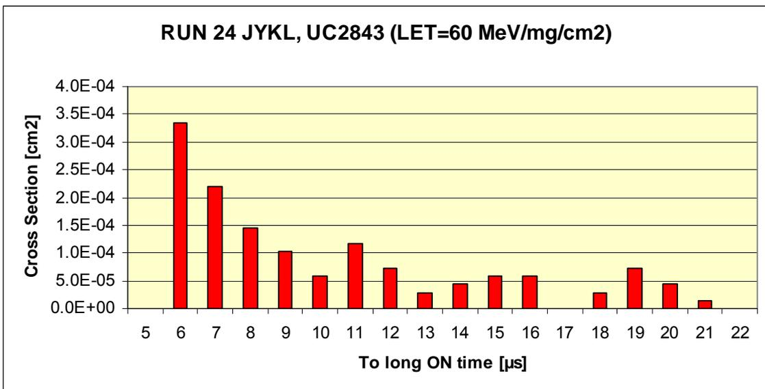
Fig 5.4.11 UC2843 histogram of too long ON time as a function of cross section.
