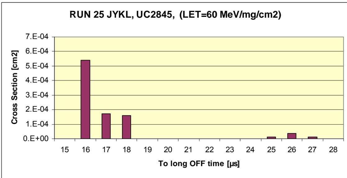
Fig 5.4.7 UC2845 histogram of too long OFF time as a function of the cross section. Irradiation in JYKL with <sup>131</sup>Xe at 0° (LET=60 MeV/mg/cm2).
