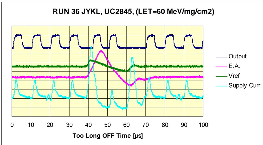
Fig 5.2.9 UC2845 Example of SET triggered by Vref
