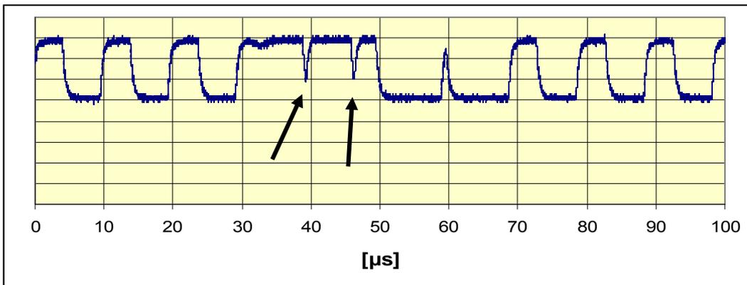
*Fig. 5.1.2 Oscilloscope graph from the output of the UC2843. The small pulse drops marked by the arrows are filtered out according to the definitions above and the "ON-time" is here calculated to be 21 $\mu$ s.*
