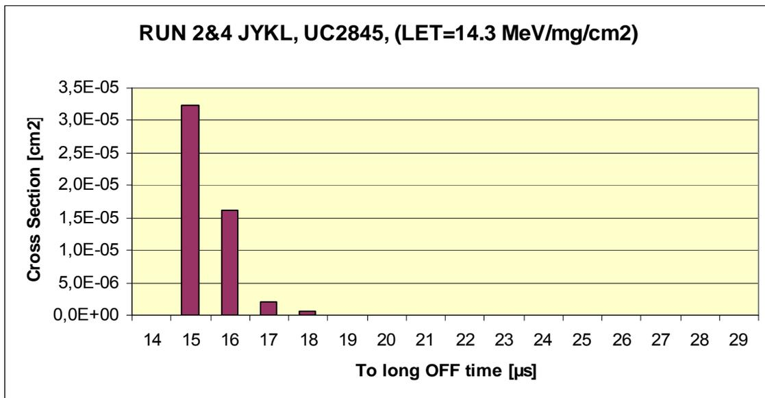
Fig 5.4.1 UC2845 histogram of too long OFF time as a function of the cross section. Irradiation in JYKL with <sup>40</sup>Ar at 45° (LET=14.3 MeV/mg/cm<sup>2</sup>).
