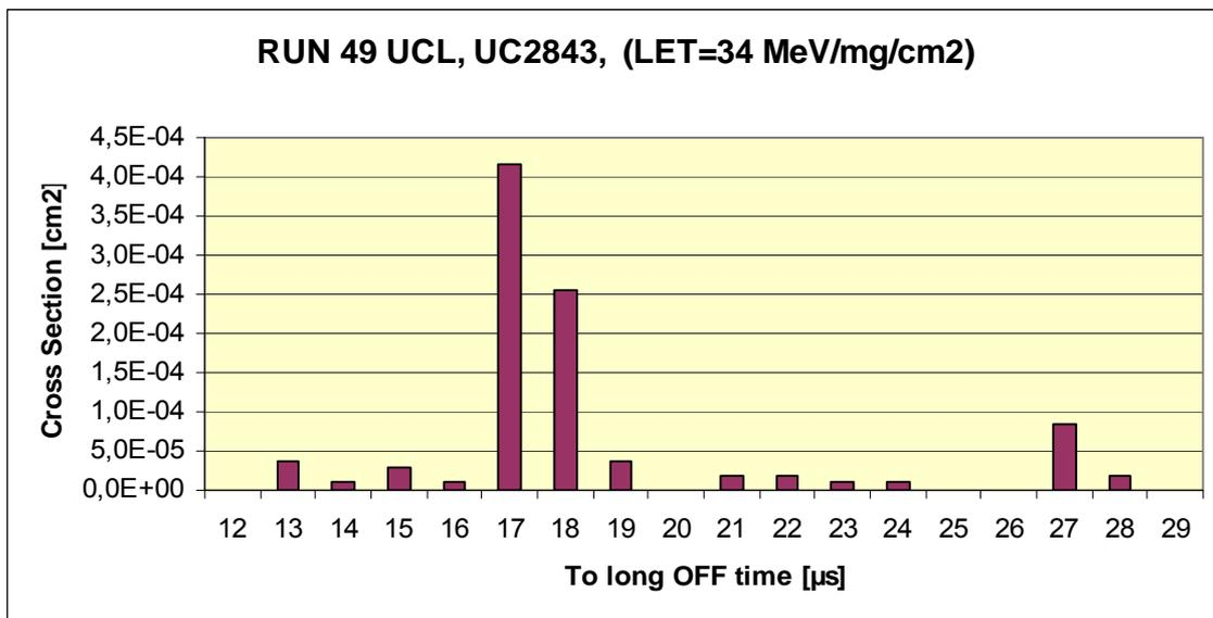
Fig 5.4.5 UC2843 histogram of too long OFF time as a function of the cross section. Irradiation at UCL with <sup>82</sup>Kr in 0° (LET=34 MeV/mg/cm2).
