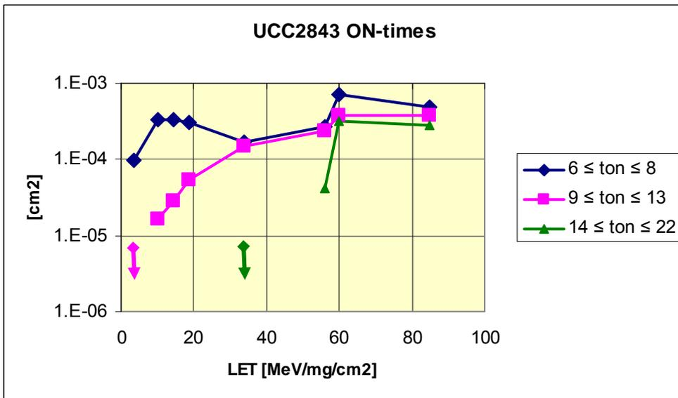
Fig 5.3.4 Too long ON time cross sections as a function of LET for UC2843.
