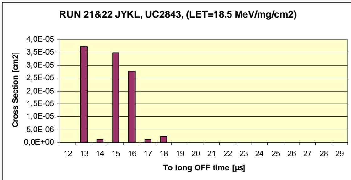
Fig 5.4.3 UC2843 histogram of too long OFF time as a function of the cross section. Irradiation in JYKL with <sup>56</sup>Fe at 0° (LET=18.5 MeV/mg/cm2).
