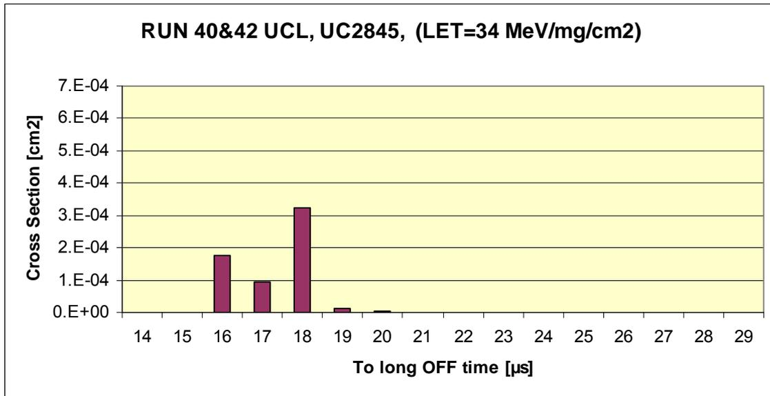
Fig 5.4.4 UC2845 histogram of too long OFF time as a function of the cross section. Irradiation at UCL with <sup>82</sup>Kr in 0° (LET=34 MeV/mg/cm2).
