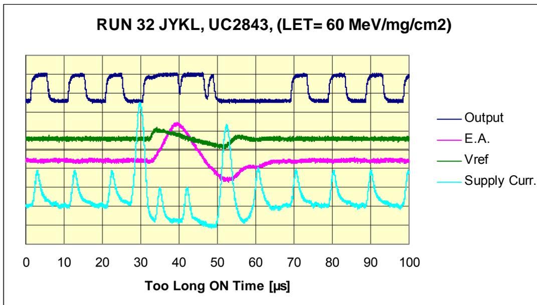
Fig 5.2.10 UC2843 @ 100kHz; Worst case SET triggered by the Output.
