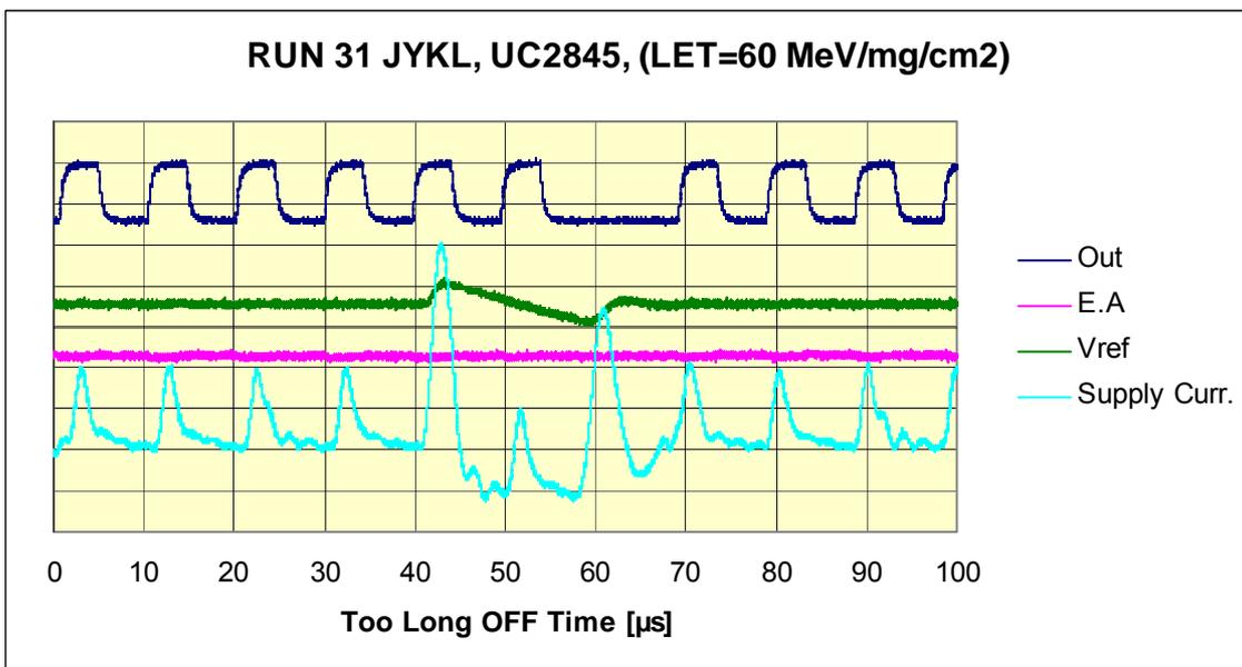
Fig 5.2.4 UC2845. Too long OFF time triggered by Output with Vref and Supply Current effected
