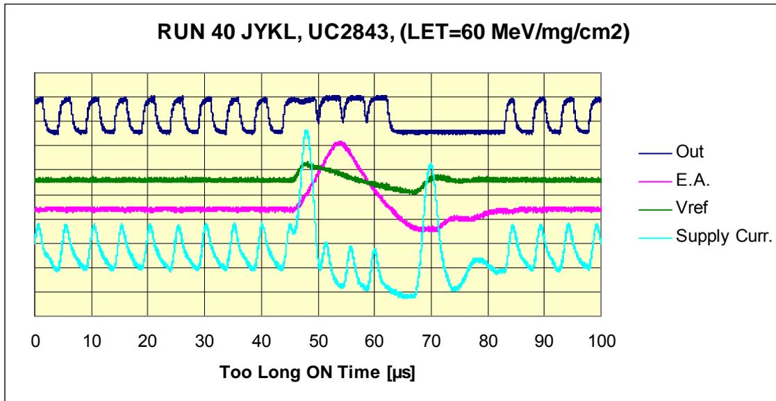
Fig 5.2.11 UC2843 @ 200 kHz; Worst case SET triggered by too long ON time on the Output. Doubling of the frequency only seem to double events affecting the duty cycle while the observed ON and OFF times are about constant in length.
