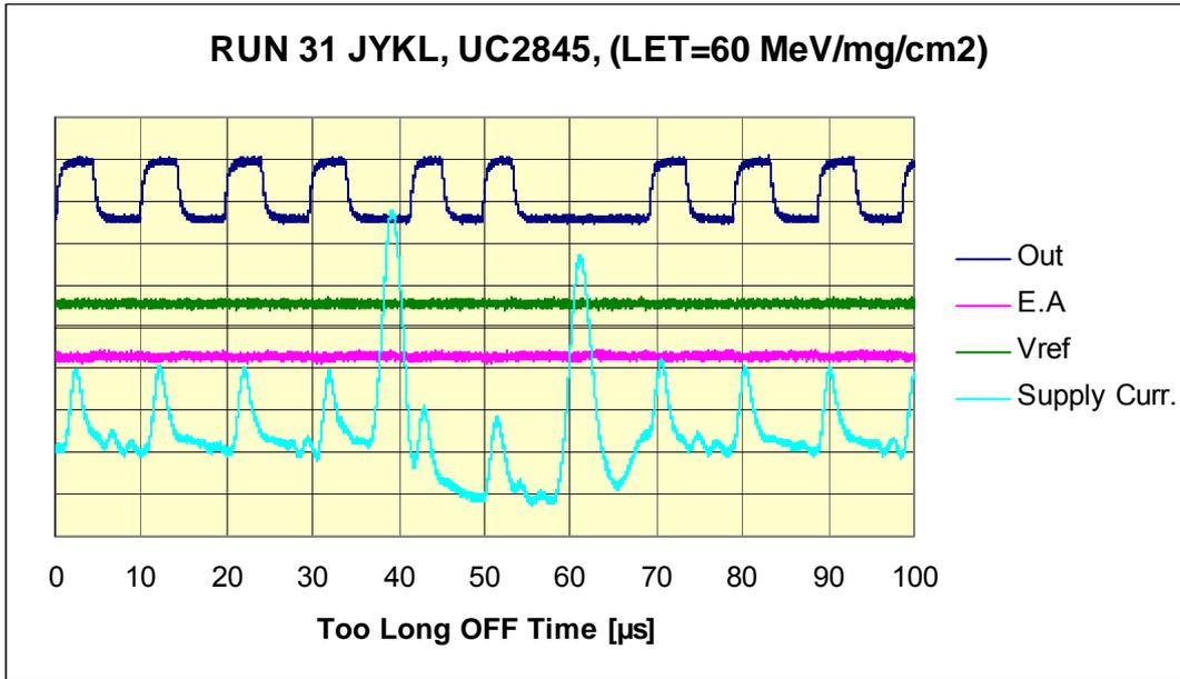
Fig 5.2.5 UC2845. Too long OFF time triggered by Output with Supply Current effected
