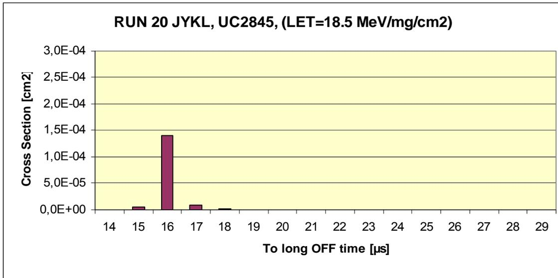
Fig 5.4.2 UC2845 histogram of too long OFF time as a function of the cross section. Irradiation in JYKL with <sup>56</sup>Fe at 0° (LET=18.5 MeV/mg/cm2).
