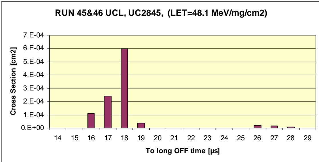
Fig 5.4.6 UC2845 histogram of too long OFF time as a function of the cross section. Irradiation at UCL with <sup>82</sup>Kr in 45° (LET=48.1 MeV/mg/cm2).
