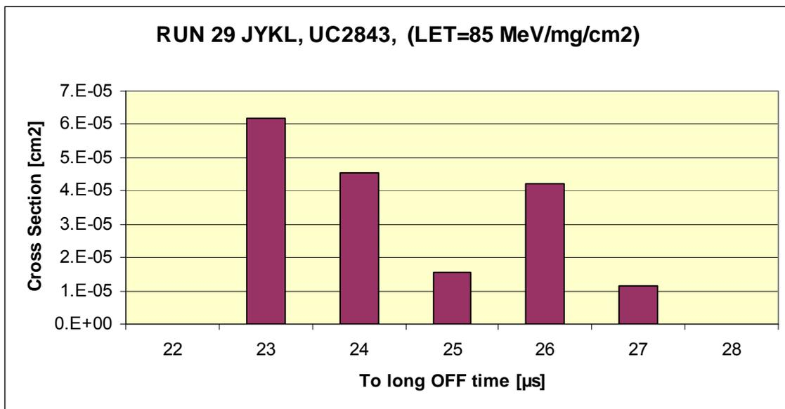
Fig 5.4.13 UC2843 histogram of too long OFF time as a function of the cross section with oscilloscope trigger conditions >22µs. The test was performed to collect better statistics on the longer OFF times. Irradiation in JYKL with <sup>131</sup>Xe at 45° (LET=85 MeV/mg/cm2).
