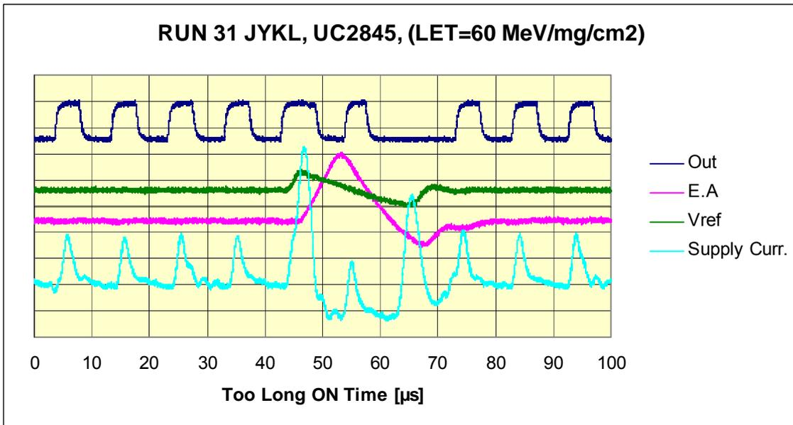
Fig 5.2.7 UC2845 Too long ON time triggered by Output. Too long ON time pulses were often followed by a too long OFF time.
