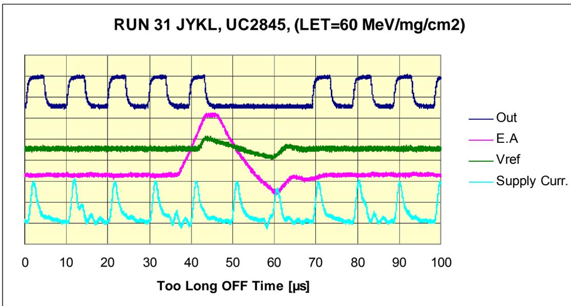
Fig 5.2.6 UC2845. Too long OFF time triggered by Output where two pulses have been missed. This oscilloscope picture represents typical SET with OFF time around 25μs.
