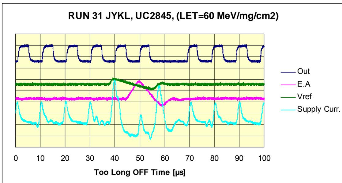
Fig 5.2.2 UC2845, Too long OFF time triggered by Output with E.A, Vref and Supply Current effected by the event.
