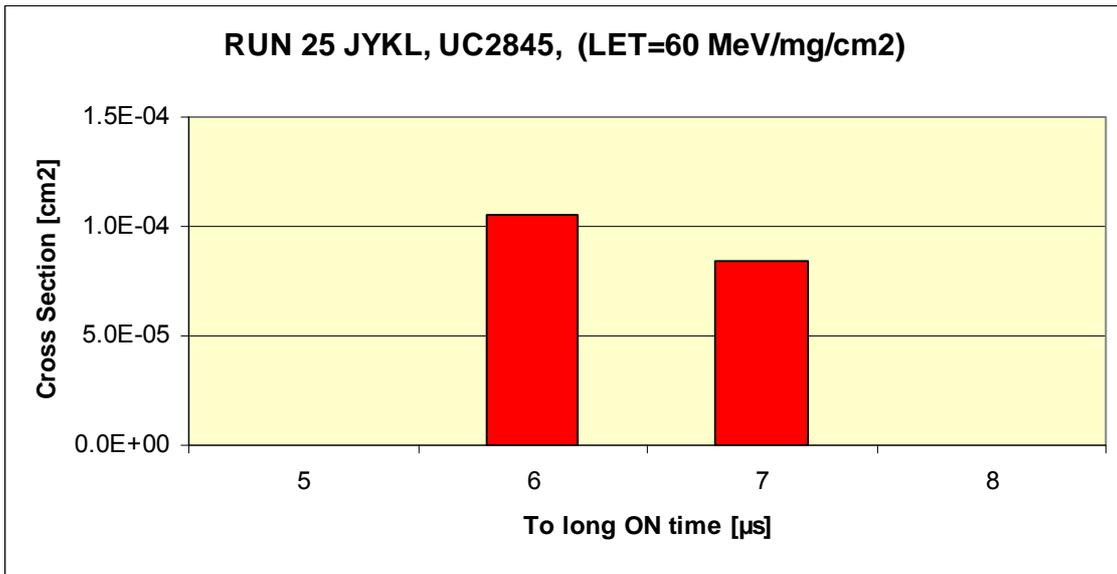
Fig 5.4.10 UC2845 histogram of too long ON time as a function of cross section.
