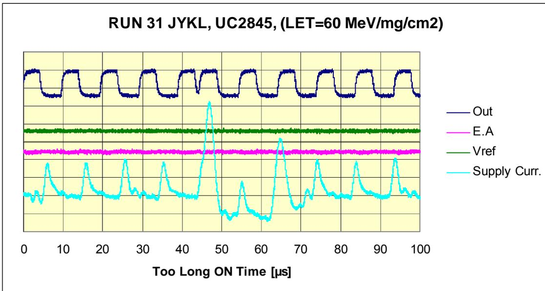
Fig 5.2.8 UC2845 Too long ON time triggered by Output. This type of event indicates a change in duty cycle for one period only.
