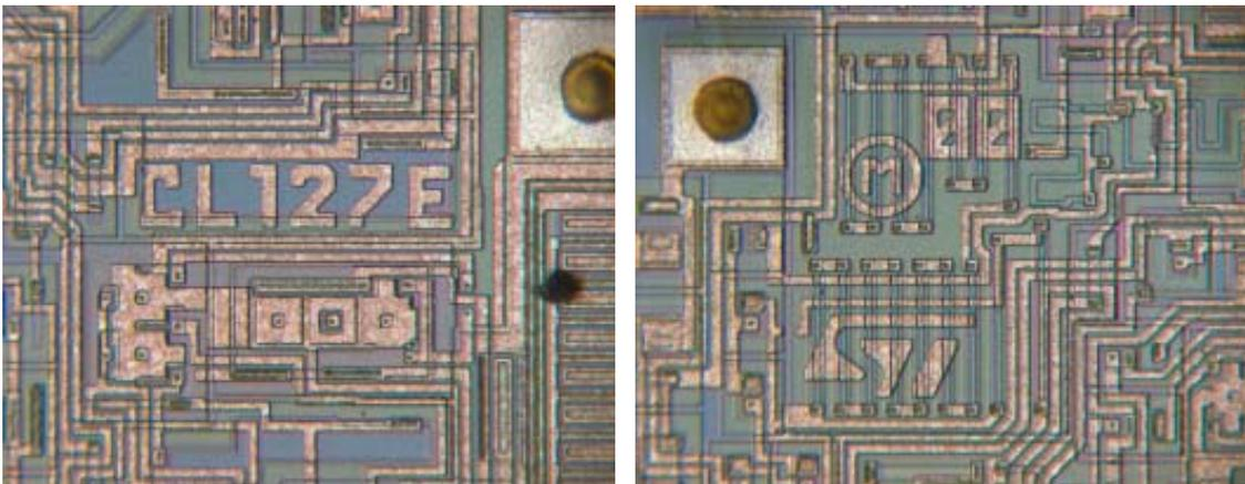
*Fig 3.1.5 Close-up picture of the chip marking on UC2845*
