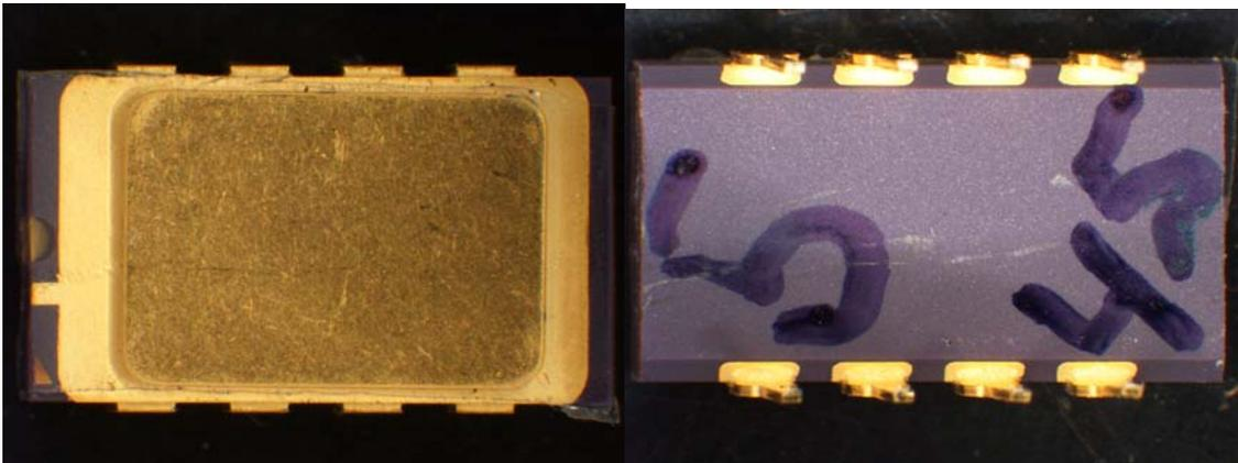
*Fig. 3.1.1 Package top & bottom view. The marking on the bottom side indicate serial number #5 and type (UC28)45.*
