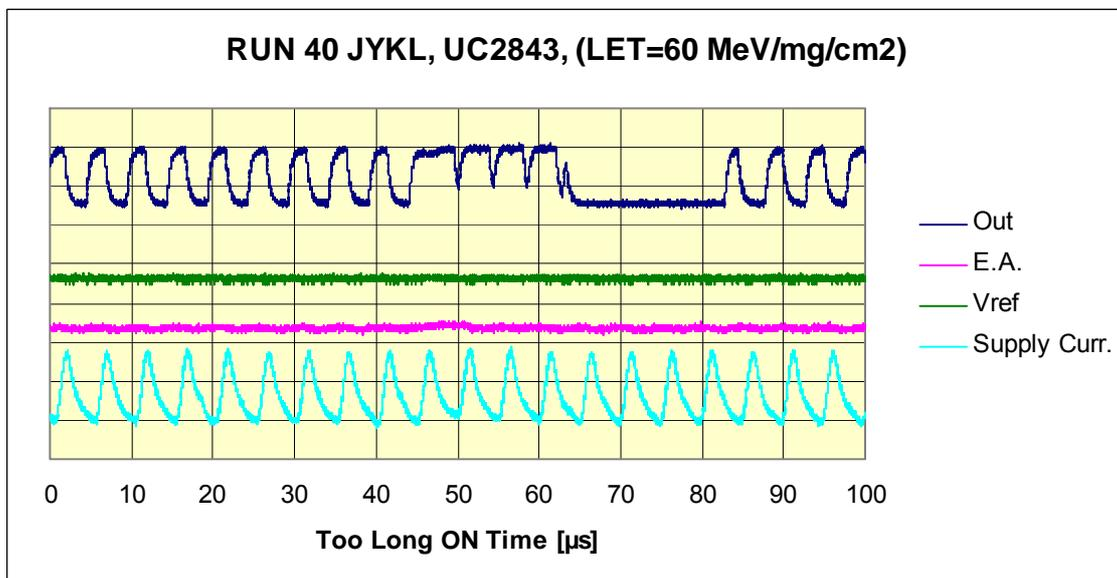
Fig 5.2.12 UC2843 @ 200 kHz; same type of Output pulse as in Fig 5.2.11 but all other signals are unaffected.
