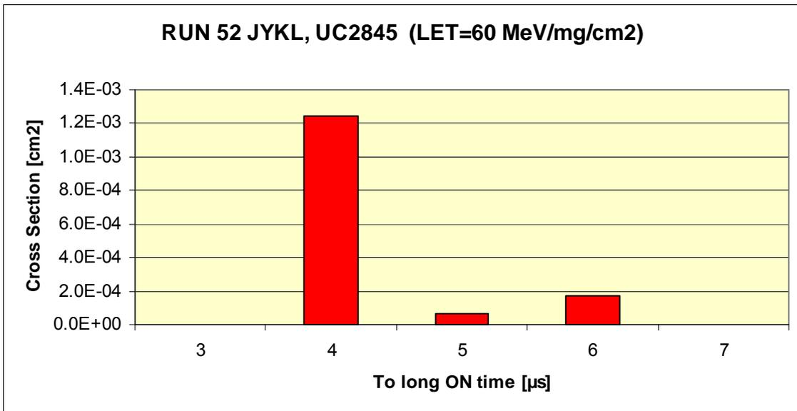
Fig. 5.4.15 UC2845 Too long ON time, Supply voltage = 20V
