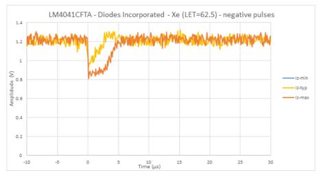
Seems like the shape of the pulse as well as its duration is more dependent on the Iz condition than on the LET.
