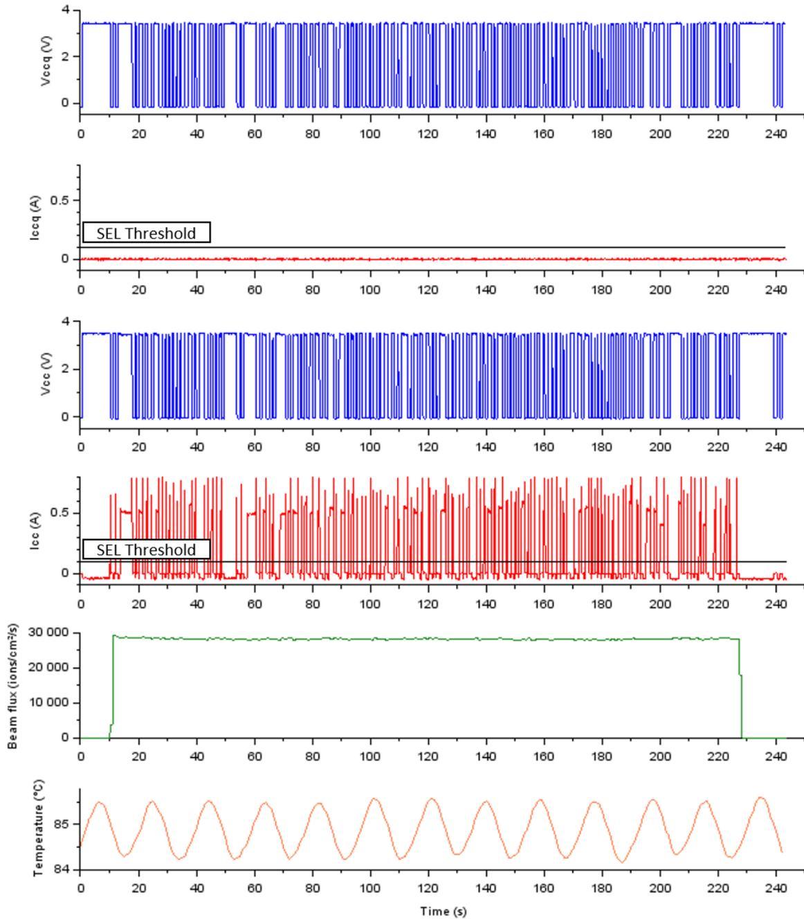
Figure 14: Campaign 1 run 92 chronograms for Vccq and Vcc lines along with temperature and flux.
