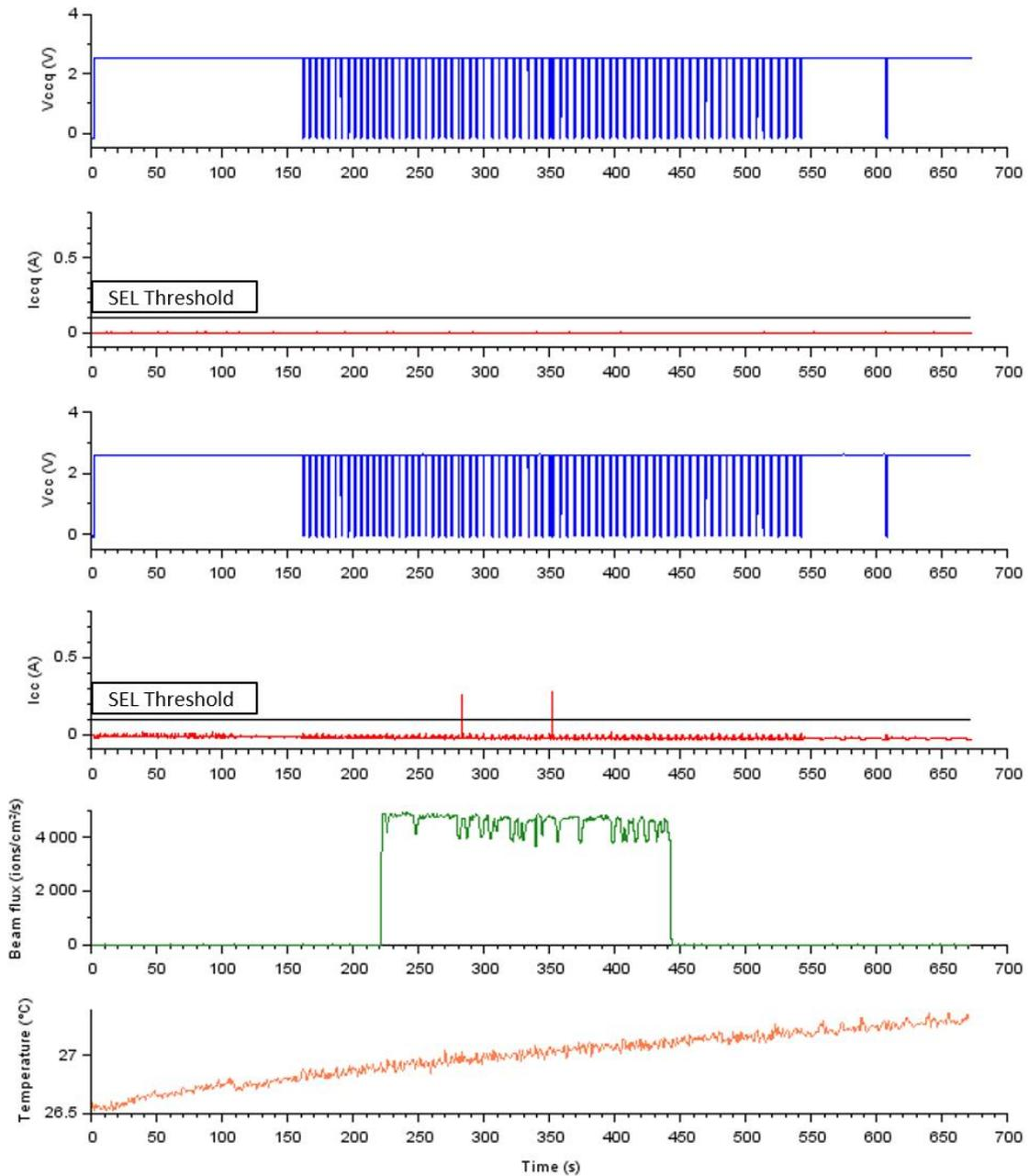
Figure 16: Campaign 2 run 41 chronograms for Vccq and Vcc lines along with temperature and flux.
