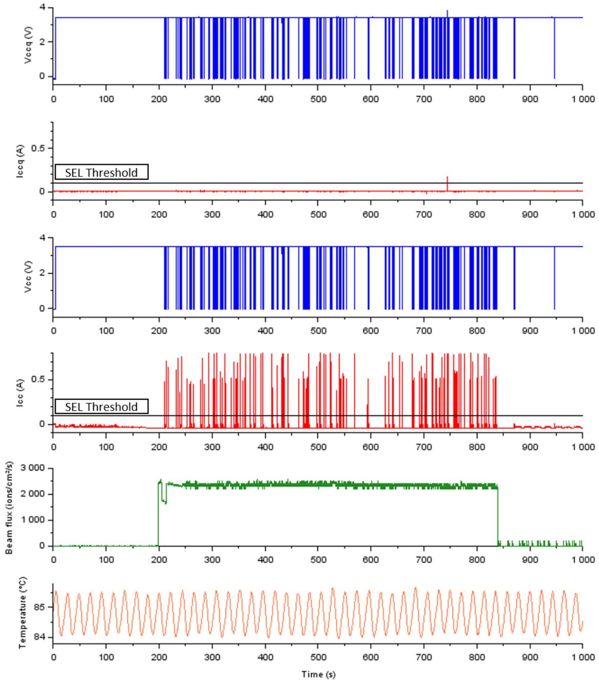
Figure 15: Campaign 2 run 44 chronograms for Vccq and Vcc lines along with temperature and flux.
