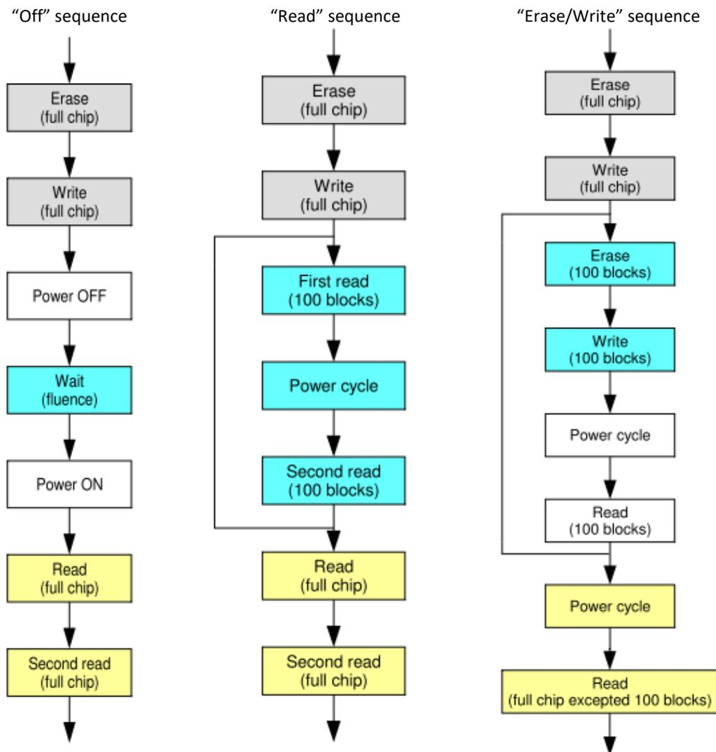
**Figure 6: Test modes used during the test campaign.**
