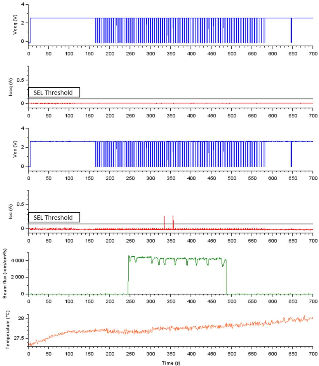
Figure 17: Campaign 2 run 42 chronograms for Vccq and Vcc lines along with temperature and flux.
