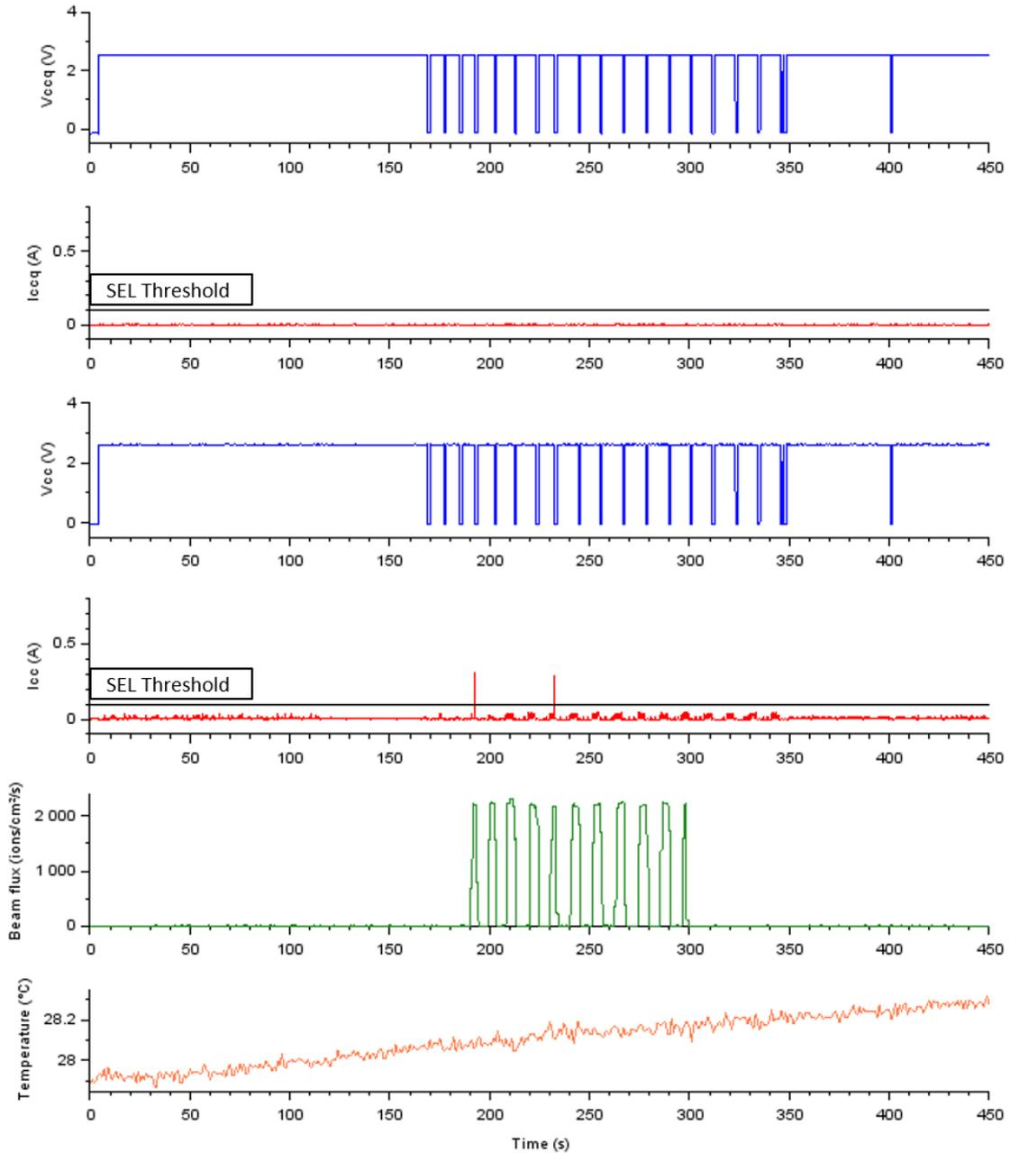
Figure 18: Campaign 2 run 43 chronograms for Vccq and Vcc lines along with temperature and flux.
