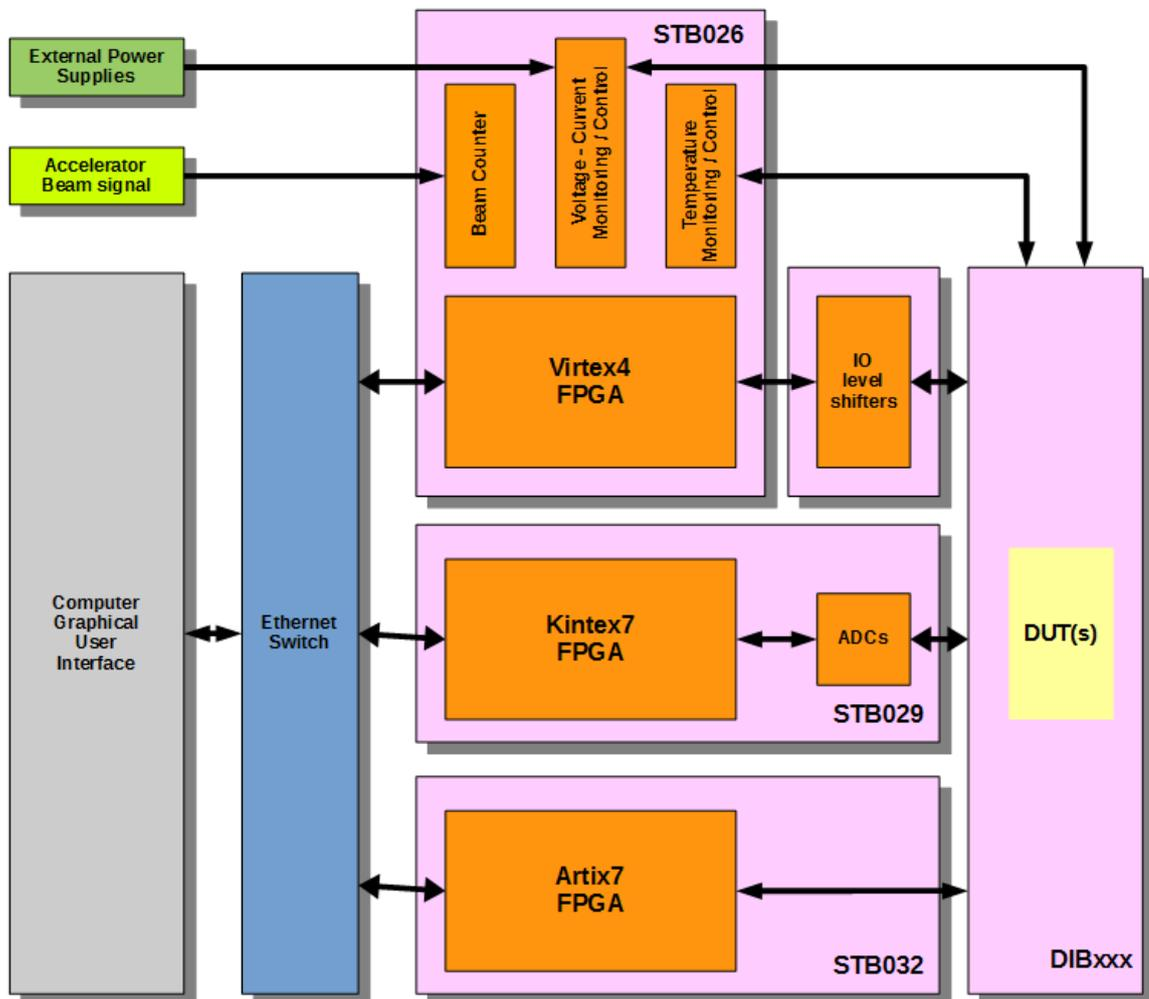
Figure 5: Hirex SEL test setup
