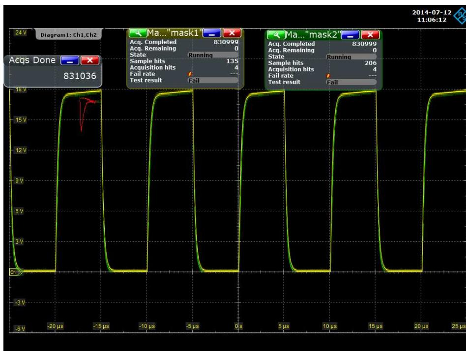
Figure 15: SET\_1, VCC=+18V, Roll 90, Heavy Ion <sup>83</sup>Kr<sup>25+</sup>, Tilt 63°, Part 14, Run n°50, Event n°5
